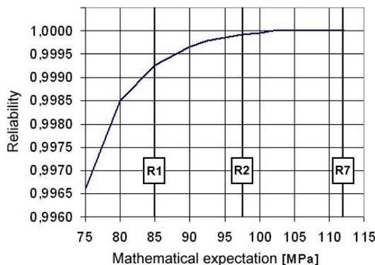
Figure 3. The influence of the wheel material limit fatigue strength mathematical expectation on the wheel reliability.
