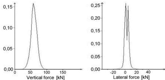
Figure 1. Vertical and lateral force empirical distributions on the wheel in the first operating regime [1].
