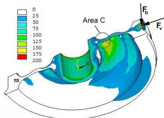
Figure 2. Wheel stress state under the effect of the vertical and lateral force (stresses are in MPa).
