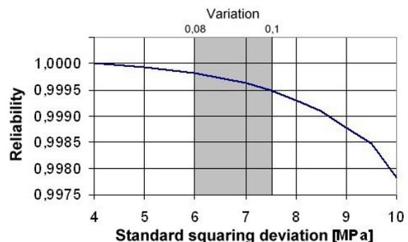
Figure 4. The influence of the wheel material limit fatigue strength standard squaring deviation on the wheel reliability
