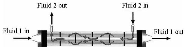
Figure 6. A fully baffled cylindrical module [3].
