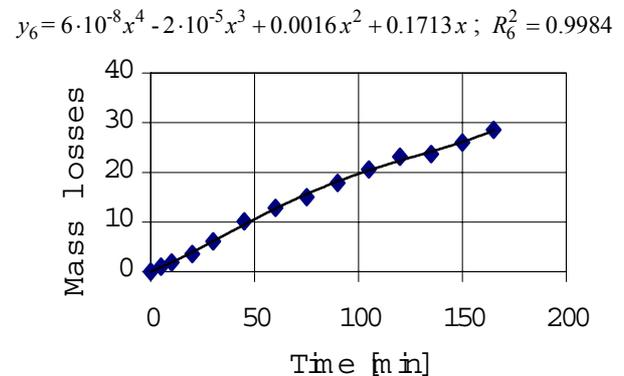
Figure 13: Specimen 6; compulsory fourth degree polynomial regression. Mass evaluation
