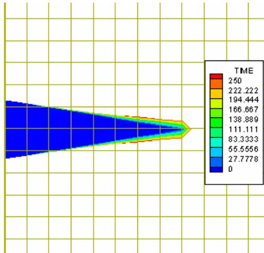
Figure 12. The front configuration of the planar edge polygonal crack until time step  $T = 250$
