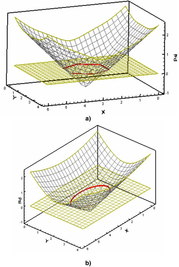
Figure 2. The distance value from 0 to 3 of LS-functions for a) polygonal and b) elliptical planar front
