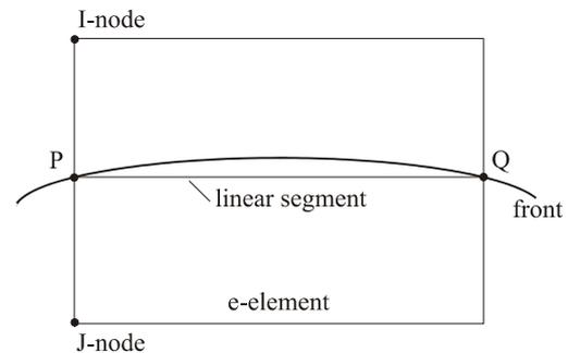
Figure 3. The linear segment of the crack on the elemente
