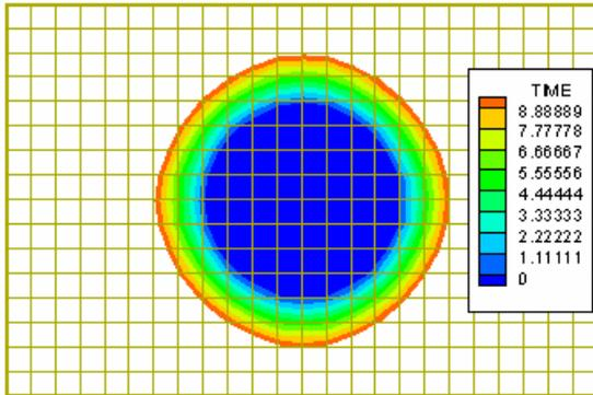
Figure 7. The arrival time of planar penny shaped crack front
