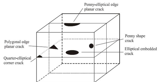
Figure 6. Typical crack shapes
