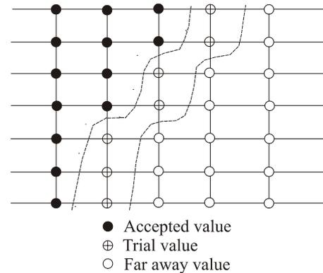
Figure 4. Upwind construction of computational domain
