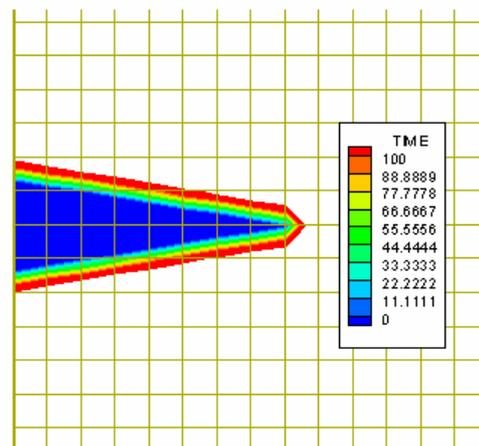
Figure 11. The arrival time of the planar edge polygonal crack
