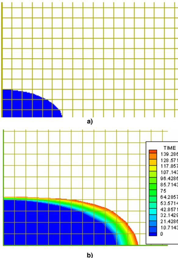
Figure 13. a) Quarter – elliptical corner crack b) Arrival time for quarter-elliptical corner crack until time step  $T = 150$
