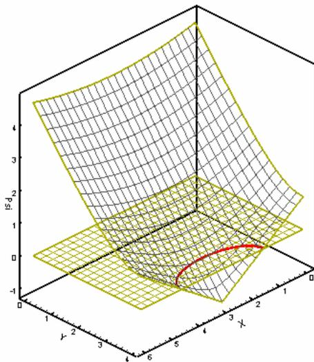
Figure 8. The signed distance level set function of the edge planar semi-elliptical crack
