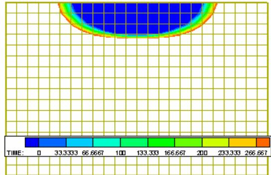
Figure 9. The front configuration semi-elliptical edge crack until time step  $T = 300$
