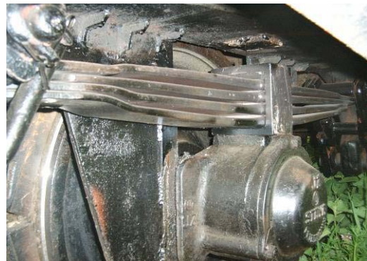
Figure 2. Spring at middle axle of DDam wagon
