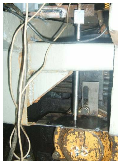
Figure 5. Mounting of displacement sensor
