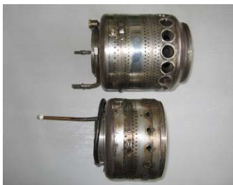
Figure 7. Photo of whole combustion chamber with Model I and without dilution zone with Model II
