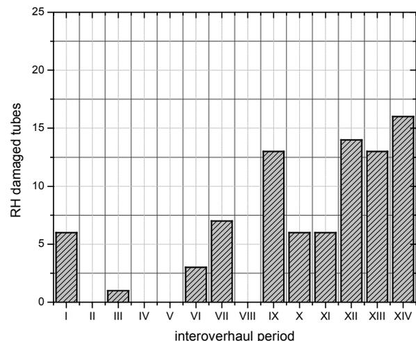
Figure 3. Number of RH damaged tubes vs. interoverhaul periods
