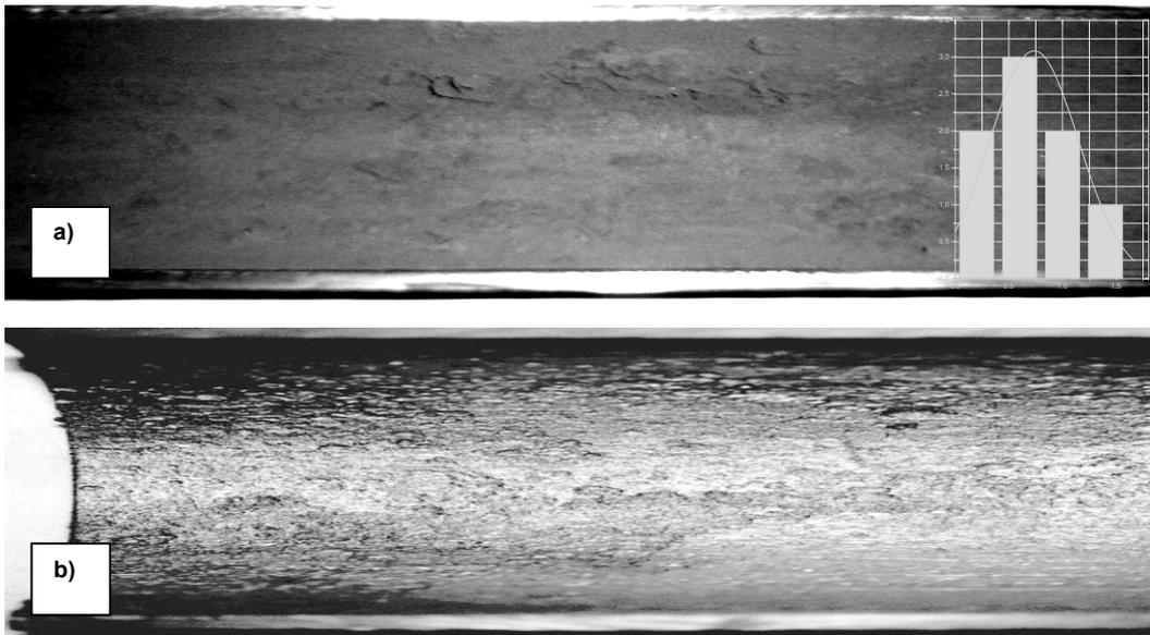
**Figure 5. Macro view of corrosion damage at the inner surface with the distribution of pit depths ( $d$ , mm: mean=0.73450; SD=0.41382). The inner surface before (a) and after removal of the deposit (b)**
