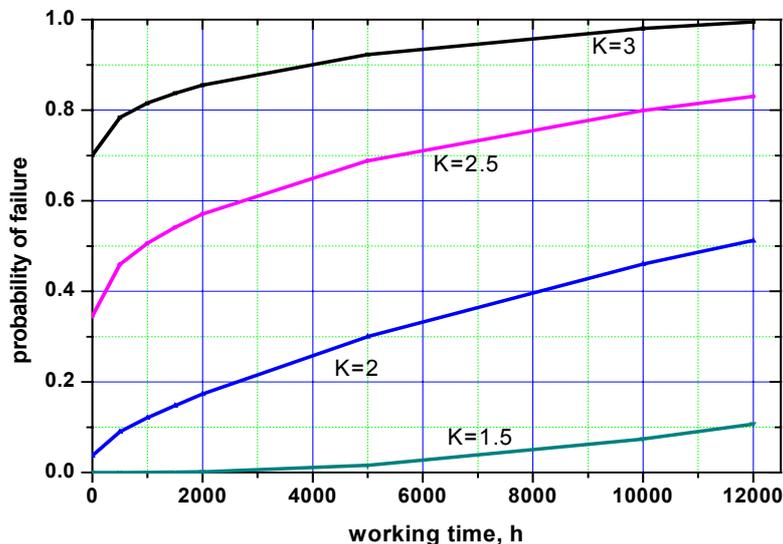
**Figure 11. Probability of failure vs. time for specified stress concentration factor K and constant corrosion rate**
