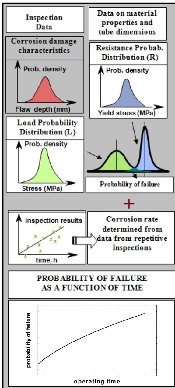
Figure 1. Algorithm for determination of PoF
