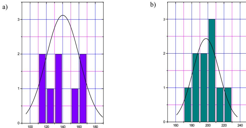
**Figure 10. Distribution of: operating stresses in the tube wall in the damaged zones [MPa] (a); distribution of flow stress at operating temperature [MPa] (b)**
