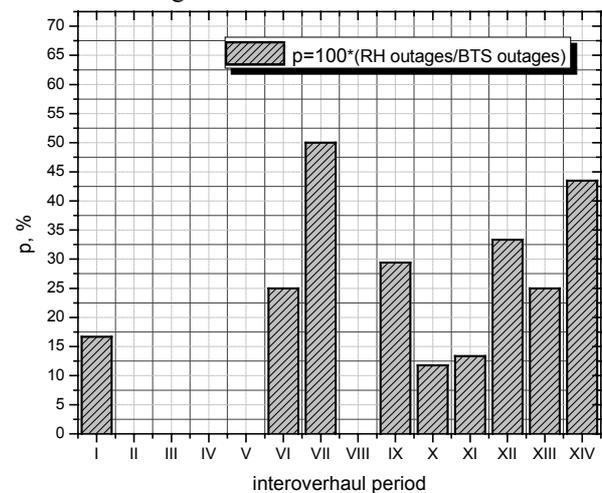
Figure 2. RH outages in comparison to the total number of boiler system (BTS) outages vs. interoverhaul periods
