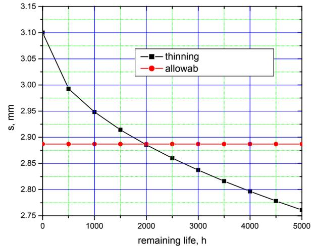
Figure 9. Remaining life of RH tube
