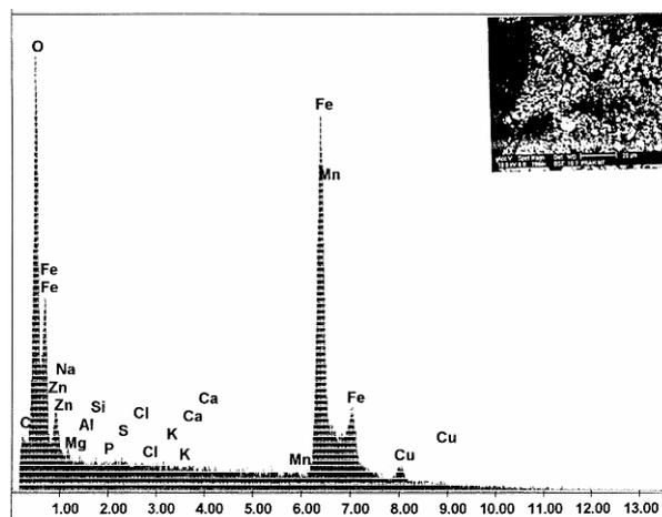
**Figure 6. EDAX of RH tube inner-side deposit**
