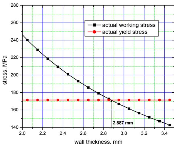
Figure 8. Actual operating stress vs. tube thickness
