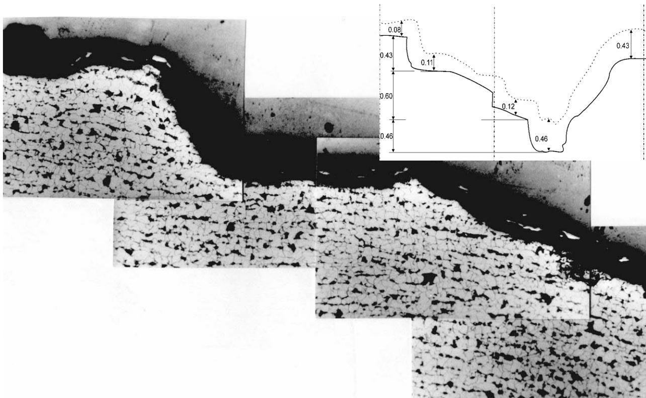
**Figure 7. Typical microstructure features of the investigated steel. Inner side. Layered ferrite-pearlite. Corrosion damage. Deposit (100x). The schematic diagram shows the entire profile of corrosion pit.**
