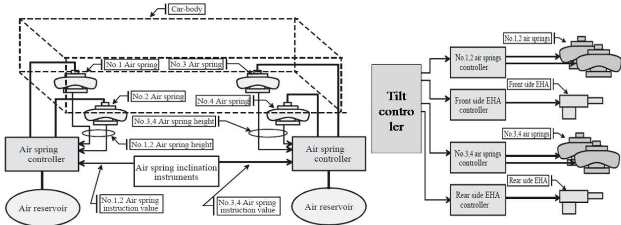
Figure 2. Model of active system of suspension on tilting train
