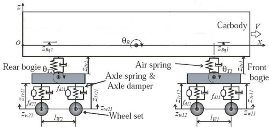
Figure 4. Classical mechanical model of tilting train [5]
