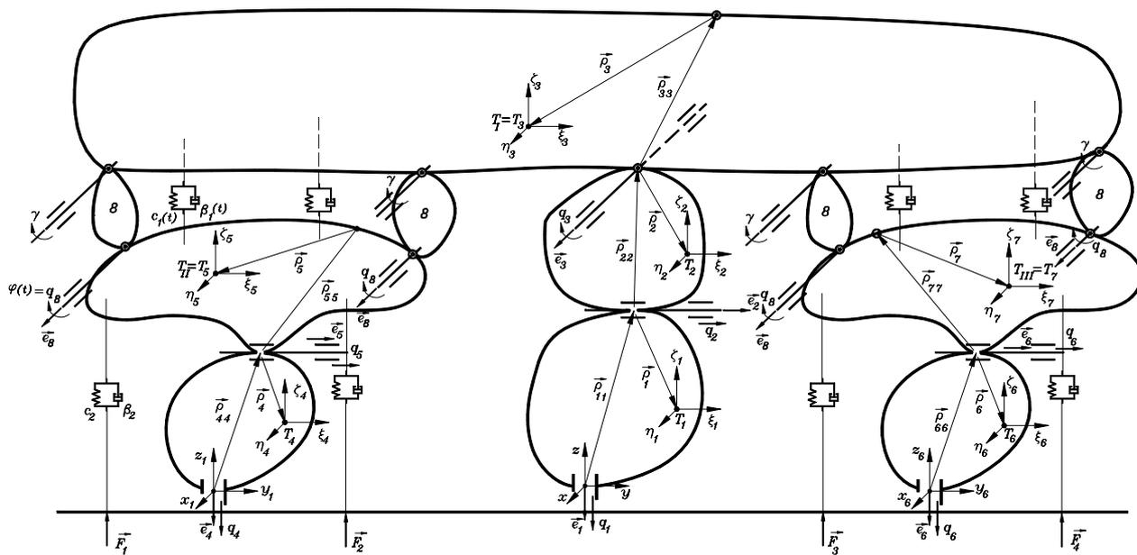
Figure 5. Advanced mechanical model of tilting train in the form of kinematical chains
