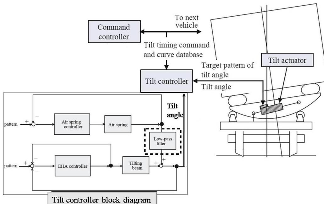
Figure 3. Controller block diagram of tilt actuator
