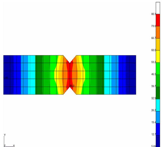
Figure 8. Stress distribution in the model
