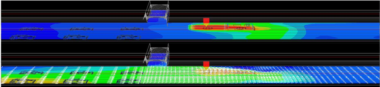
Figure 6. Air velocity and smoke concentration field at the height of  $z = 2$  m, in case of a fire caused by a bus on fire, at maximum air flow rate determined for the ventilation of the tunnel, for the distance of 90 m between the ventilators and evacuation openings
