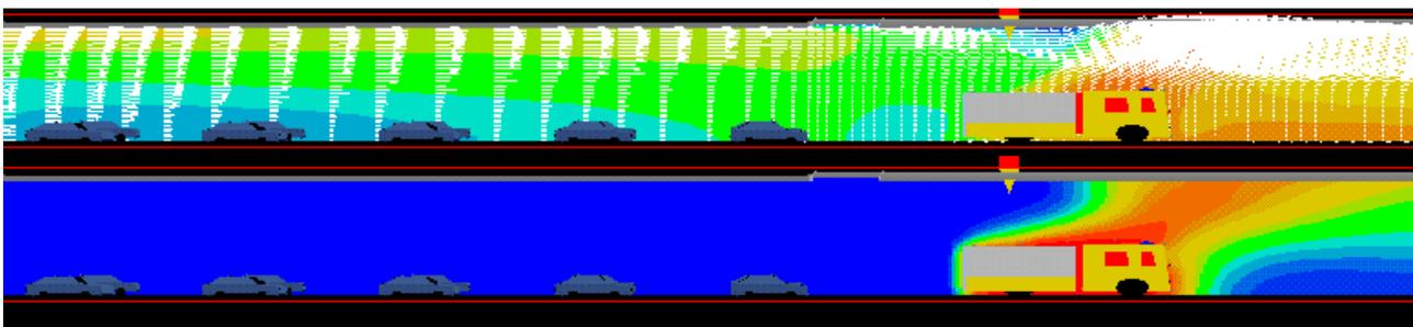
Figure 7. Smoke concentration field on the plane  $x = 3$  m from the axis of the tunnel, in case of a fire caused by a bus on fire, at 1.6 times higher air flow rate than the maximum determined for the ventilation of the tunnel, for the distance of 90 m between the ventilators and evacuation openings
