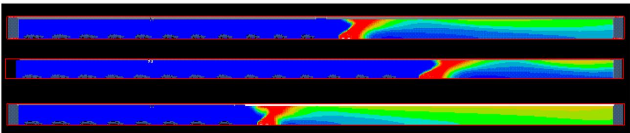
Figure 3. Smoke concentration field on the plane  $x = 3 \text{ m}$  from the axis of the 250 m long part of the tunnel, in case of a fire caused by a passenger vehicle on fire, at maximum air flow rate determined for the ventilation of the tunnel, for three distances of 30, 60 and 90 m of the ventilators from the evacuation openings
