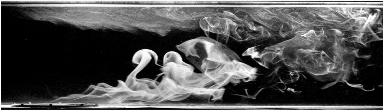
Figure 1. Photograph of a spread of smoke in a tunnel for the 15 kW fire [4]
