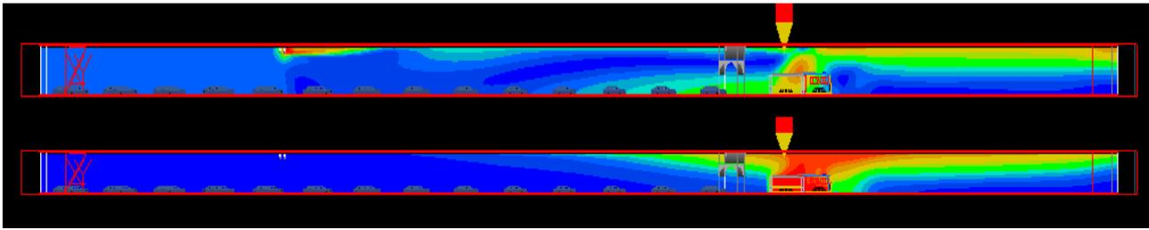
Figure 5. Air velocity and smoke concentration field on the plane  $x = 3$  m from the axis of the tunnel, in case of a fire caused by a bus on fire, at maximum air flow rate determined for the ventilation of the tunnel, for the distance of 90 m between the ventilator and evacuation openings
