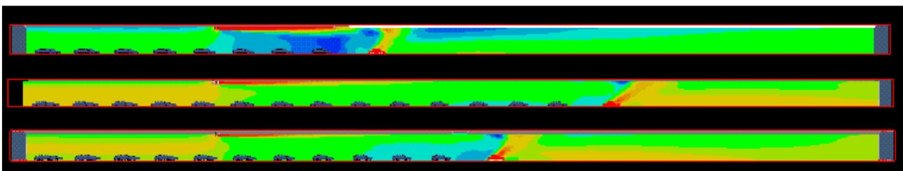
Figure 4. Air velocity field on the plane  $x = 3 \text{ m}$  from the axis of the tunnel, in case of a fire caused by a passenger vehicle on fire, at maximum air flow rate determined for the ventilation of the tunnel, for three distances of 30, 60 and 90 m of the ventilators from the evacuation openings
