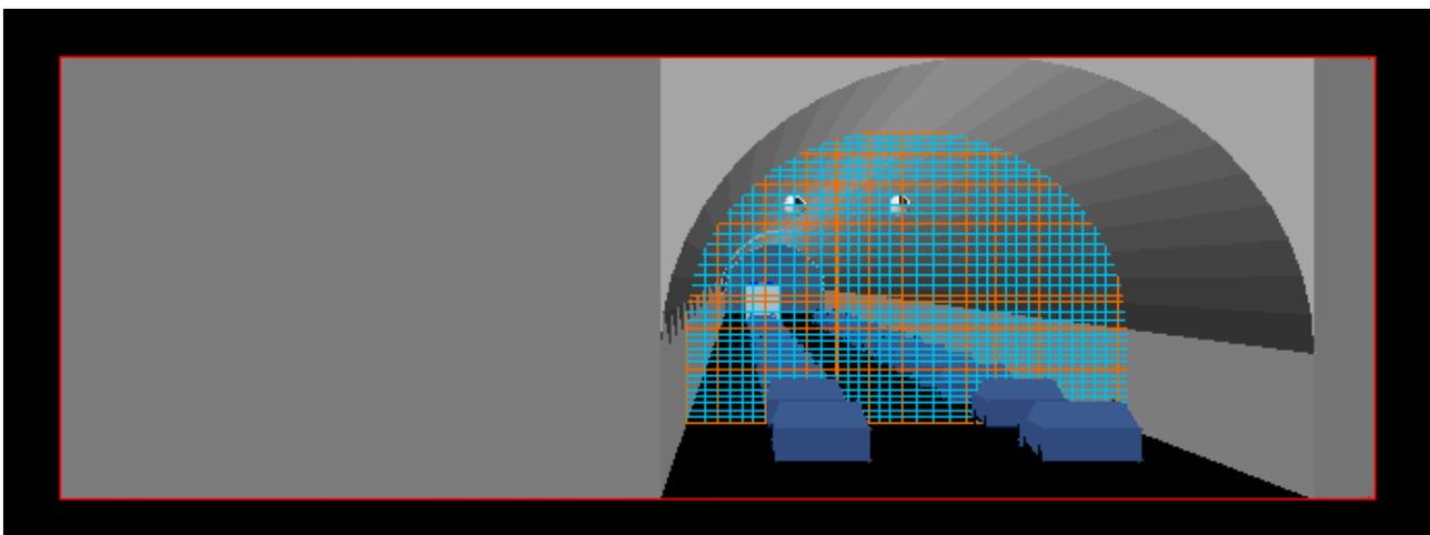
**Figure 2. Mesh of control volumes in virtual tunnel space**
