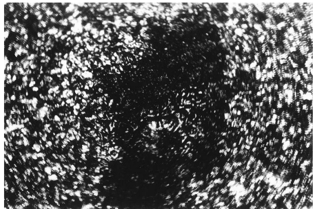
Figure 2. Micrograph of the Ni-alloy damage by TEA CO 2 laser, Spot 2; 120 pulses; E per pulse = 85 mJ; 200X
