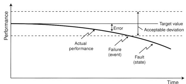
**Figure 1. Illustration of the difference between failure, fault and error [3]**
