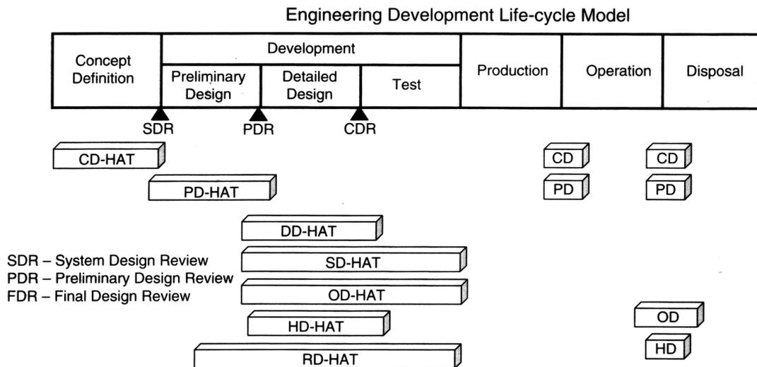
Figure 5. Overall timing of hazard analysis types
