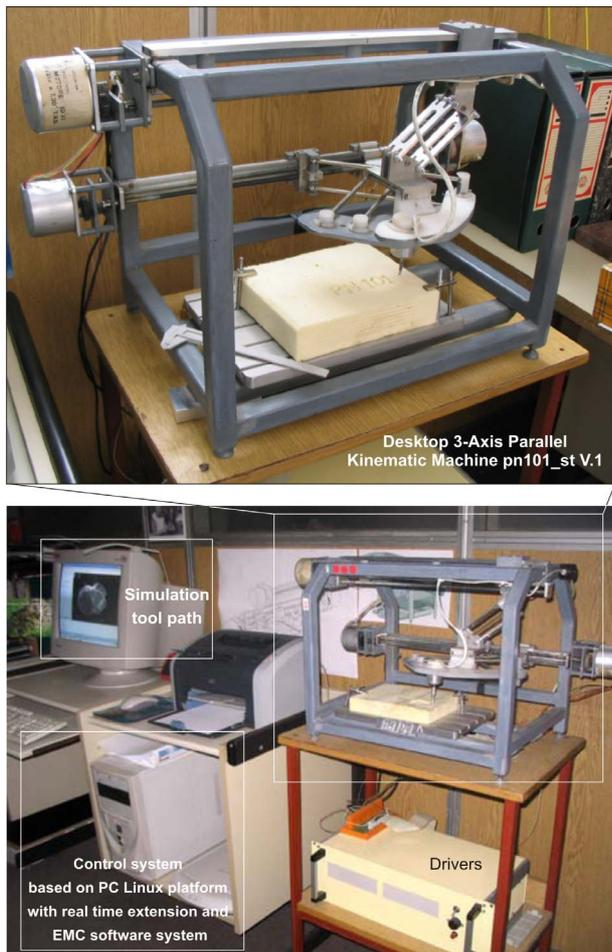
Figure 12. Desktop 3-axis parallel kinematics machine, first prototype pn101\_st V.1
