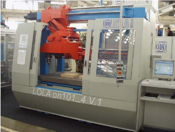
Figure 4. Experimental vertical milling machine, first industrial prototype LOLA pn101\_4 V.1 [7]
