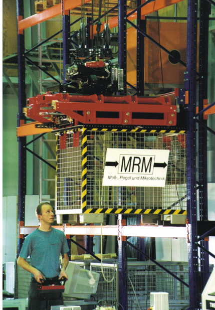
Figure 2. Example of automated handling of pallet boxes by a rope guided material handling system [6]
