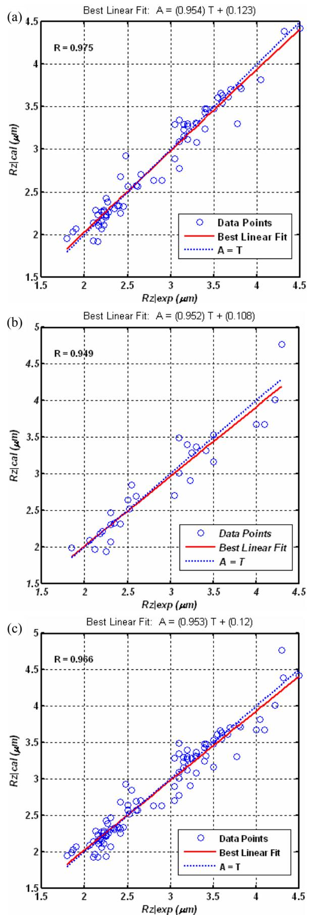
Figure 3. The performance of ANN model for surface roughness in plasma cutting process: (a) for training data set, (b) for testing data set and (c) for whole data set; The ANN was trained without noise ( $R_{z,cal}$ ). The experimental values ( $R_{z,exp}$ ) are values without noise
