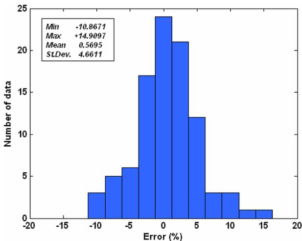
**Figure 6. Distribution of the percentage error ( $\delta$ ) for modelling the surface roughness ( $R_z$ ) in plasma cutting process**
