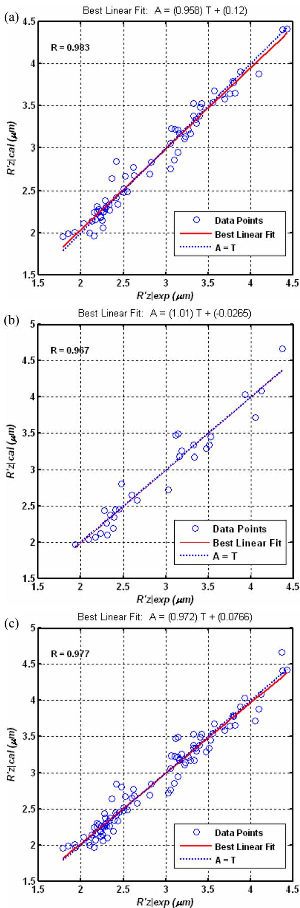
Figure 4. The performance of ANN model for surface roughness in plasma cutting process: (a) for training data set, (b) for testing data set and (c) for whole data set; The ANN was trained with added noise ( $R'_{zcal}$ ). The experimental values ( $R'_{zexp}$ ) are values including noise
