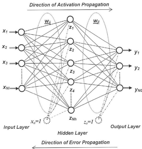
Figure 1. Topology of a typical feed-forward three-layer BP ANN
