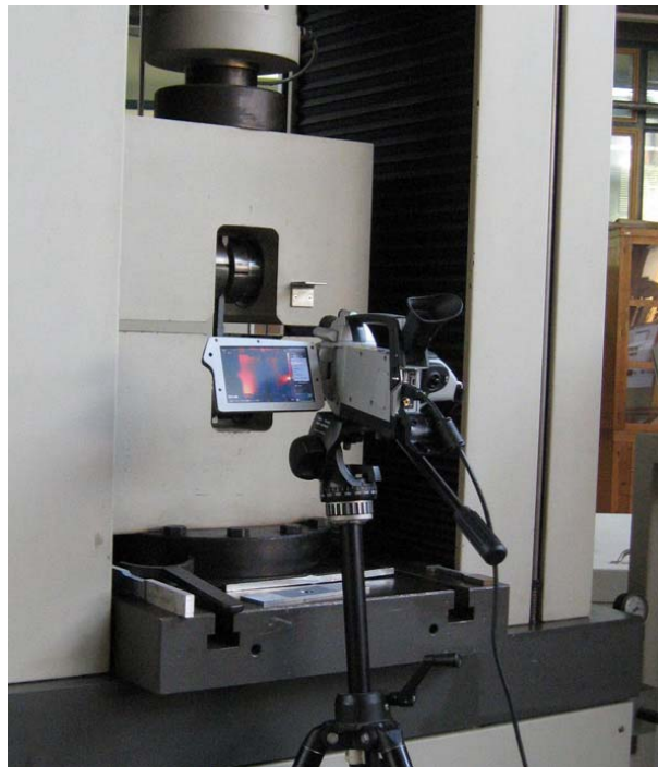
Figure 1. Tension test and thermography equipment
