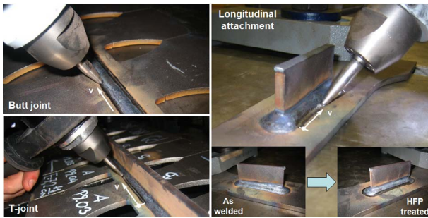
Figure 2. HFP treatment of the investigated specimens
