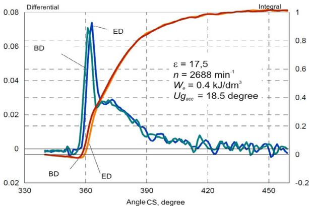
Figure 4. Integral and differential combustion rate for biodiesel and commercial diesel fuel at full load, for engine speed  $2688 \text{ min}^{-1}$  [14, 15].
