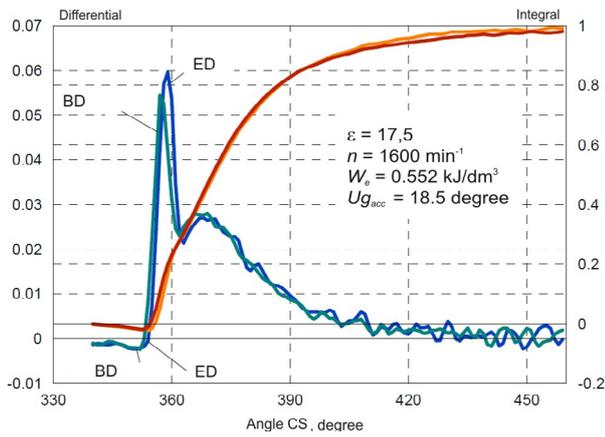
Figure 3. Integral and differential combustion rate for biodiesel and commercial diesel fuel at full load, for engine speed  $1600 \text{ min}^{-1}$  [14, 15].
