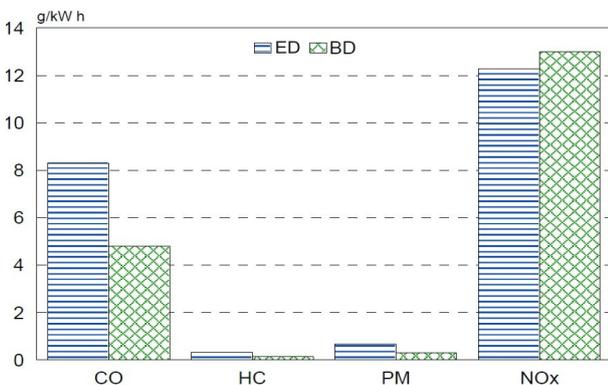
Figure 5. The values of emission of toxic components obtained by the European Steady-state Cycle (ESC), for engine operating with compression ratio of 17.5, with ED and BD [14, 15].
