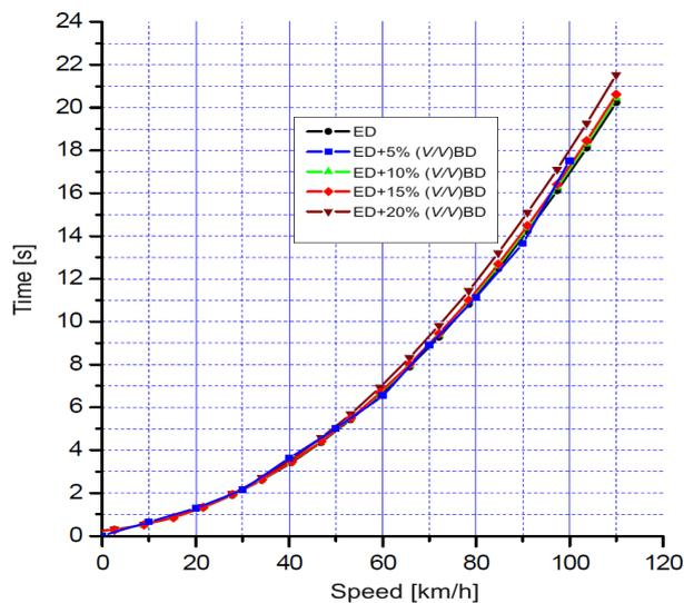
Figure 8. Vehicle acceleration from 0 to 100 km/h
