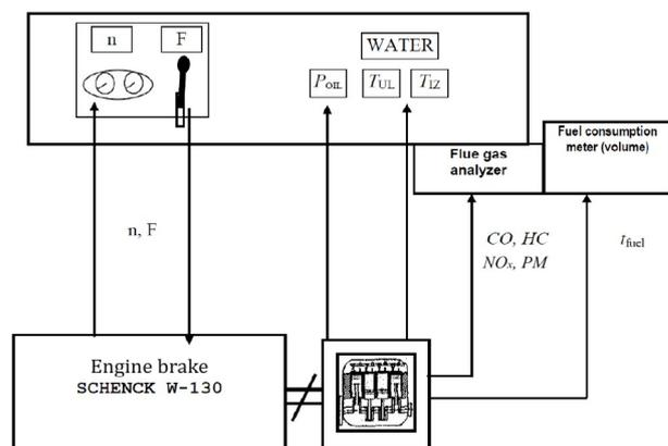
Figure 1. Schematic view of measuring and test installation
