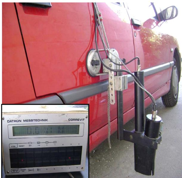
**Figure 2. Measuring system Datron for recording vehicle performances**
