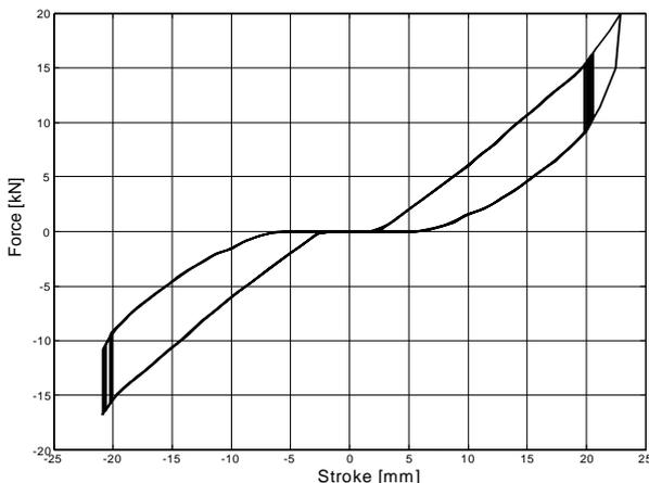
Figure 7. Force stroke characteristic based on experimental data defined in Fig. 3
