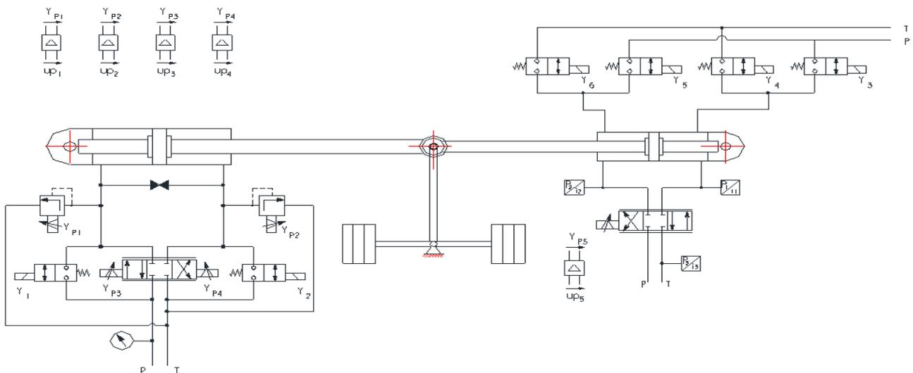
**Figure 18 Functional schematic view of test system for electro-hydraulic actuator with flexible load**
