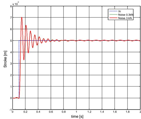
Figure 14. Position response for noise frequency 50 rad/s
