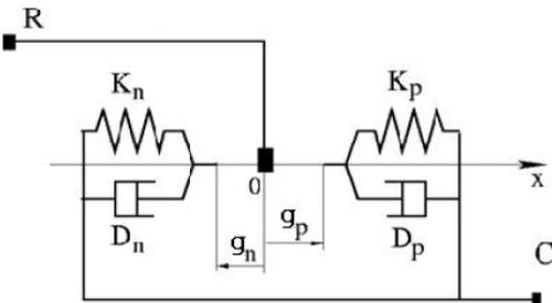
Figure 11. Mathematical structure model of non-ideal spring according to the general viscous-elastic model in Mat Lab. [15]
