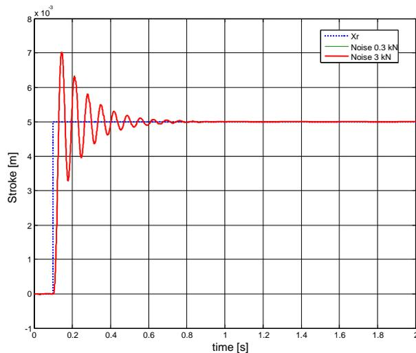
Figure 13. Position response for noise frequency 20 rad/s
