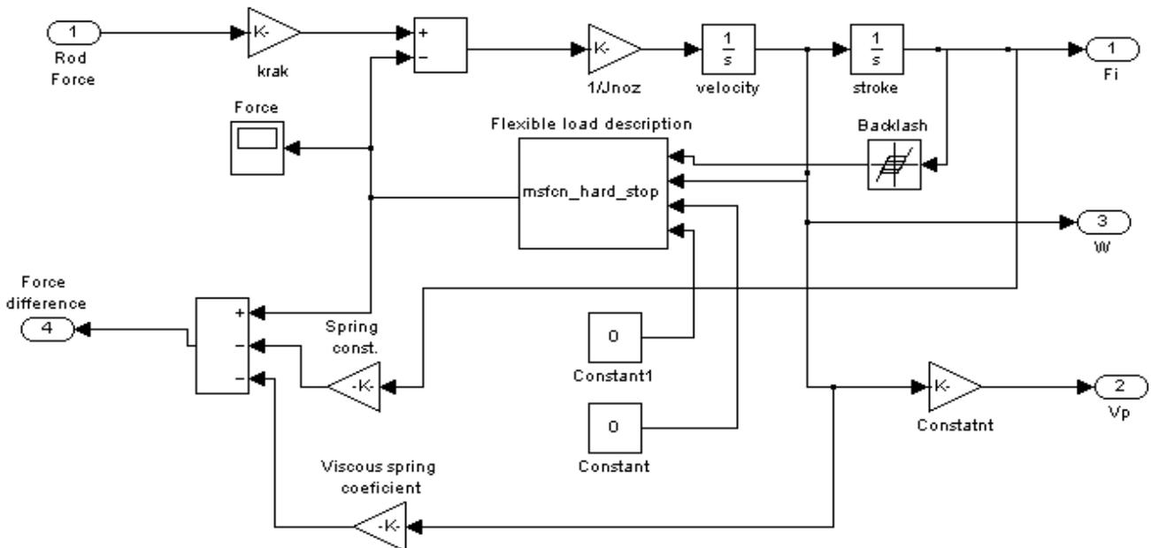
Figure 10. The structure of mathematical model for load simulation
