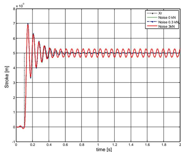
Figure 15. Position response for noise frequency 90 rad/s
