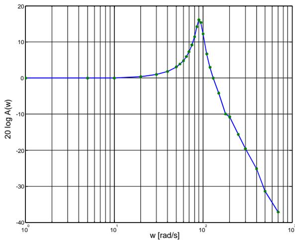
**Figure 17. Amplitude characteristic of actuators closed loop system**
