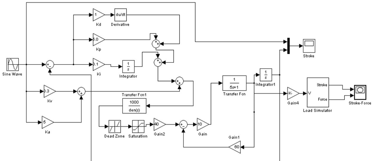
Figure 5. Block diagram of actuator control system with flexible load
