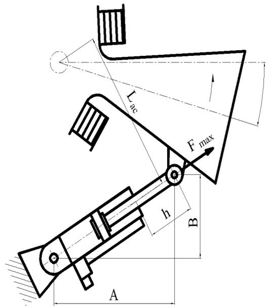
**Figure 1. Basic schematic view of a flexible nozzle construction**
