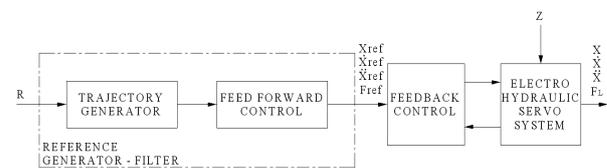
**Figure 4. Structural schematic view of actuator control configuration [10]**
