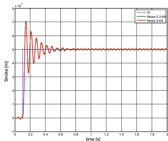
Figure 16. Position response for noise frequency 130 rad/s
