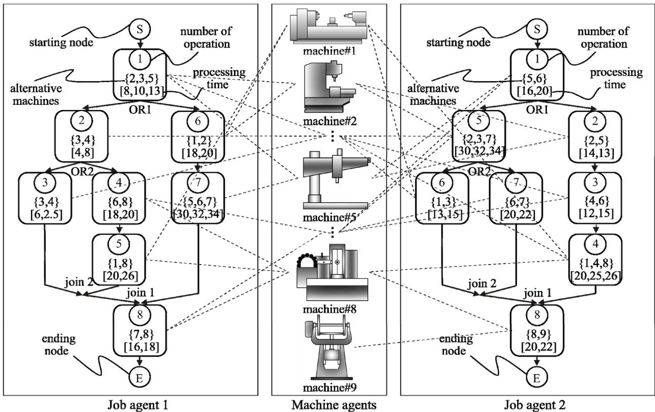
Figure 2. Alternative process plan network for two parts and nine machines
