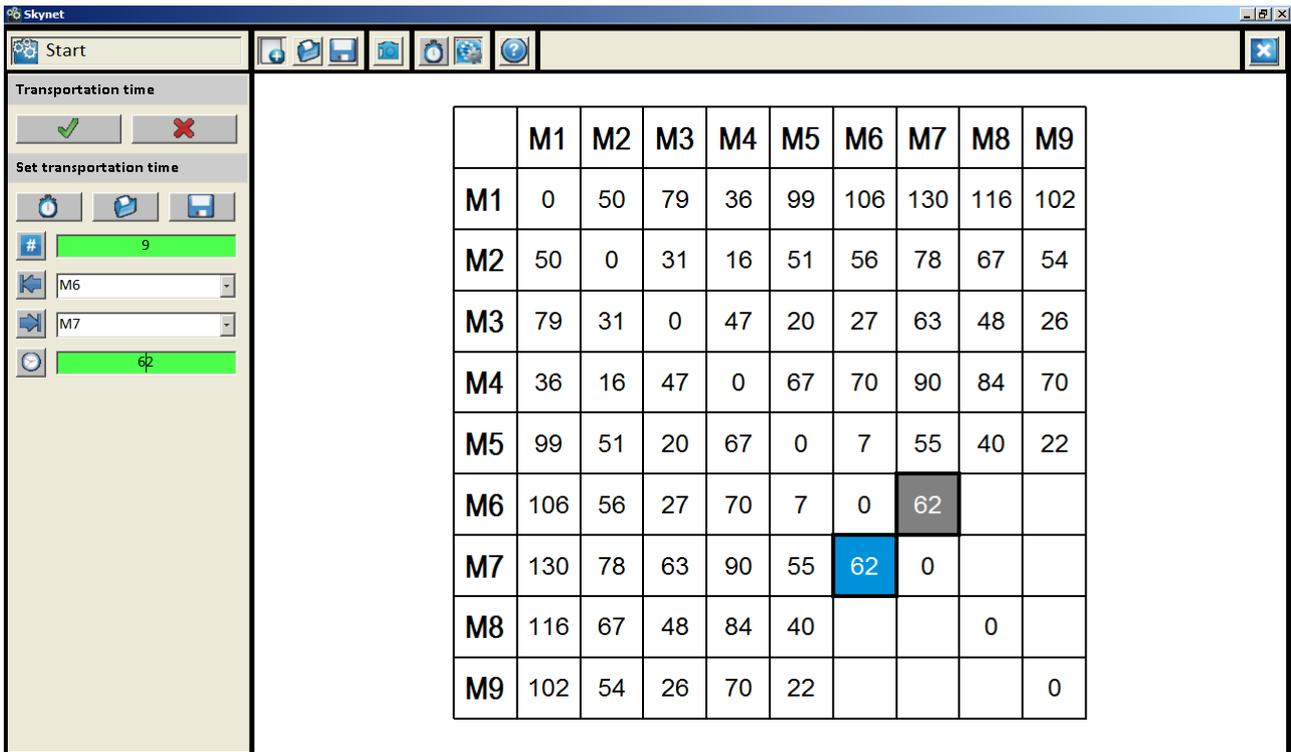
Figure 5. Machine agent: Setting transportation times between machines
