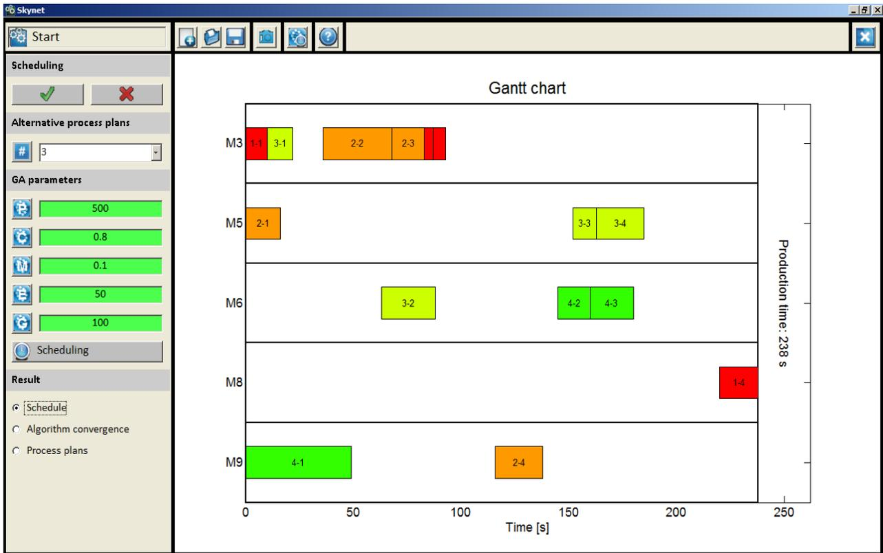
Figure 7. Optimization agent: Scheduling results for 4 jobs and 9 machines. Gantt chart is based on object 1 (Makespan=238)
