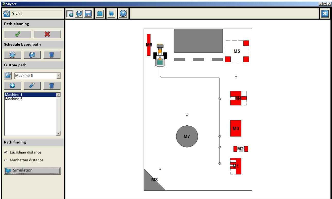
Figure 10. Path planning agent: Optimal path from machine 1 to machine 6 that mobile robot follows
