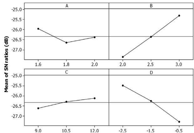
**Fig. 1. Main effect plot of S/N ratios for the width of HAZ**
