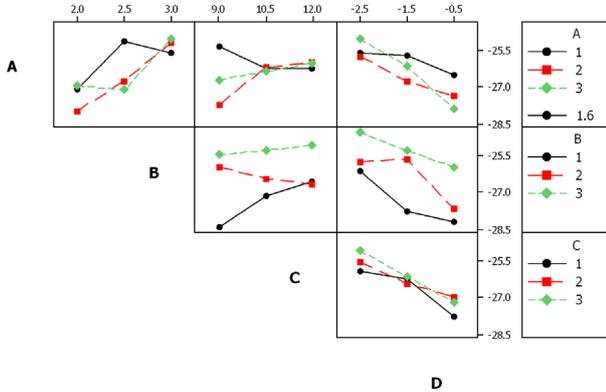
Fig. 2. Interaction effect plots of average S/N ratios for the width of HAZ
