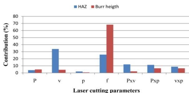
Fig. 5. Percentage contribution of the laser cutting parameters on the width of HAZ and burr height
