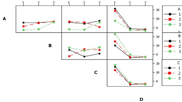
Fig. 4. Interaction effect plots of average S/N ratios for the burr height
