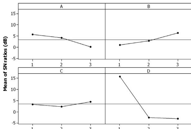
Fig. 3. Main effect plot of S/N ratios for the burr height
