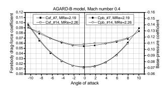
Figure 8. Repeatability check: AGARD-B model, drag-force and base-pressure coefficients, Mach 0.4
