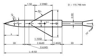
Figure 2. AGARD-B standard model – Overall geometry
