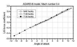
Figure 12. Inter-facility correlation: AGARD-B model, liftforce coefficient, Mach 0.4
