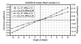
Figure 10. Repeatability check: AGARD-B model, lift-force and pitching-moment coefficients, Mach 0.4
