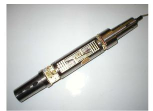
Figure 4. VTI-produced internal six-component straingauge monoblock balance
