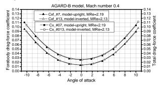
Figure 6. Test section symmetry check: AGARD-B model, forebody and total drag-force coefficients, Mach 0.4
