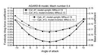
Figure 5. Test section symmetry check: AGARD-B model, drag-force and base-pressure coefficients, Mach 0.4
