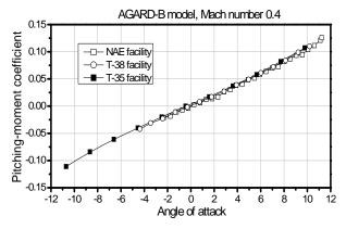
Figure 13. Inter-facility correlation: AGARD-B model, pitching-moment coefficient, Mach 0.4
