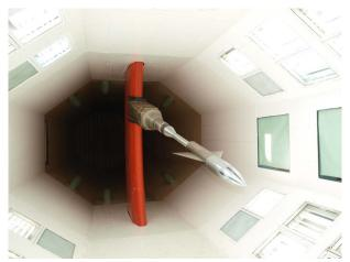
Figure 3. AGARD-B standard model mounted in the T-35 test section
