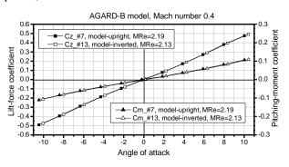
Figure 7. Test section symmetry check: AGARD-B model, lift-force and pitching-moment coefficients, Mach 0.4
