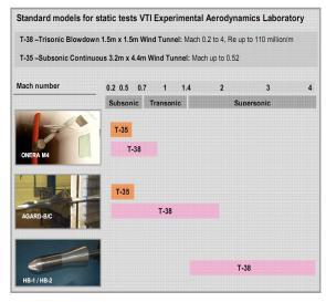
Figure 1. Mach number ranges of standard models used in VTI for static tests
