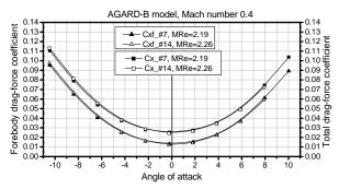
Figure 9. Repeatability check: AGARD-B model, forebody and total drag-force coefficients, Mach 0.4
