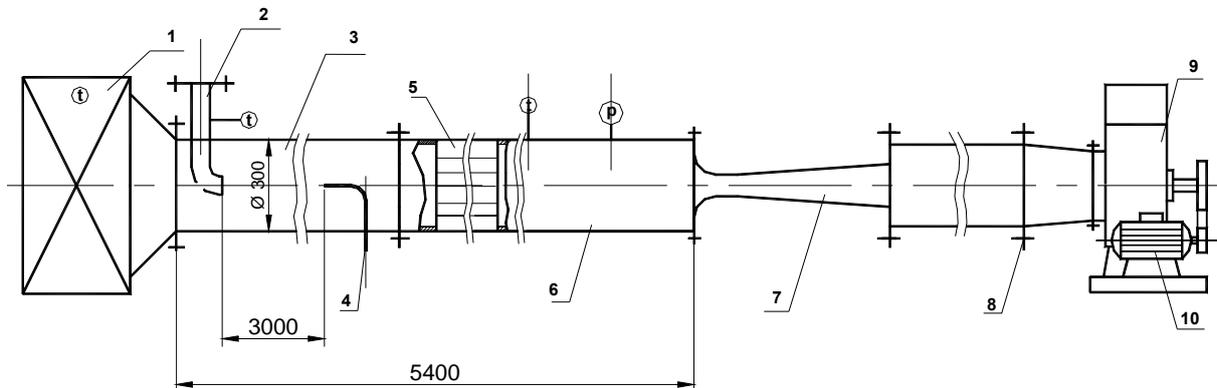
Figure 2. Drawing of a full-flow dilution tunnel [8]
