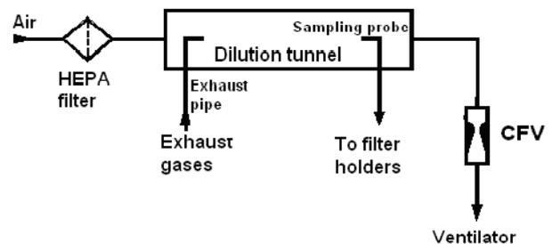
Figure 1. Schematic of a full-flow dilution tunnel
