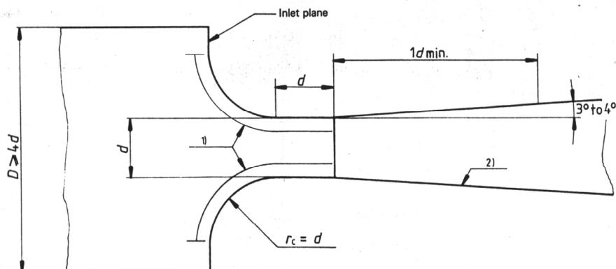
Figure 7. A drawing of a typical critical flow Venturi with a cylindrical nozzle throat [4]
