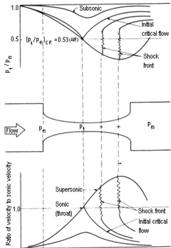
Figure 6. Pressures and fluid velocities for a Venturi nozzle [7]
