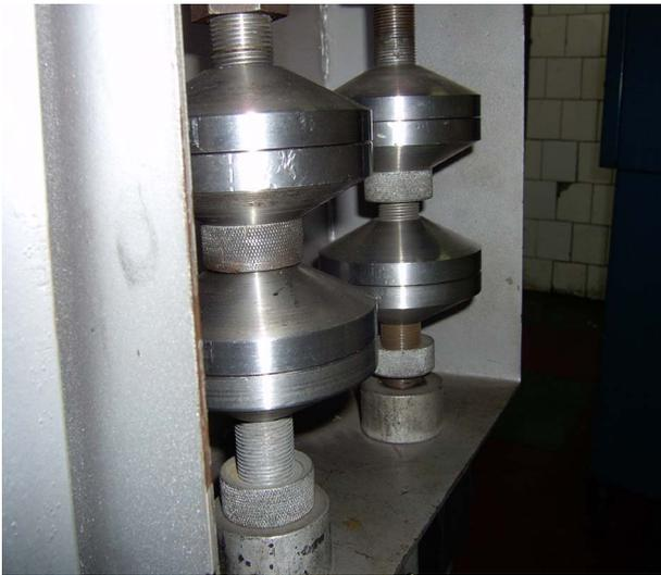
Figure 5. Filter holders for particle collection
