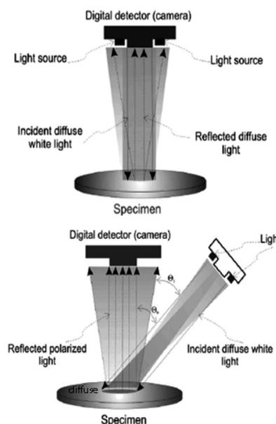
**Figure 1. Incident white light will give different information about sample surface properties, when reflected, depending on the angle of incidence. Each type of matter is characterized with a specific angle of incidence [21].**
