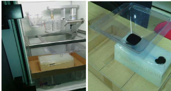
Figure 6: The casting process in a vacuum chamber MK-Technology
