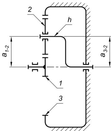
Figure 7. Coaxiality of the planetary gearbox shafts
