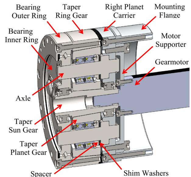
Figure 11. Planetary gearbox with taper gears - cross section
