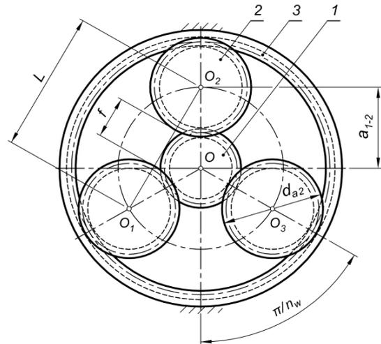
Figure 8. Displacement of the planet gears in the main plane of the planetary gearbox
