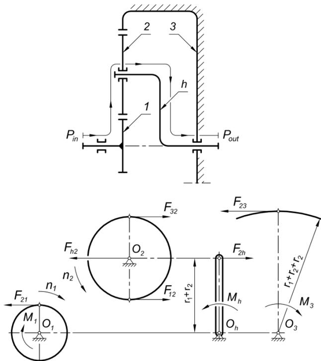
Figure 9. Power flow, forces and torques acting upon elements of the planetary gearbox
