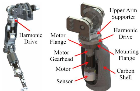
**Figure 2. Design of robot's arm and robot's upper arm**
