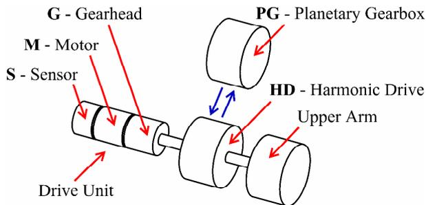
Figure 5. Drive system of the upper arm
