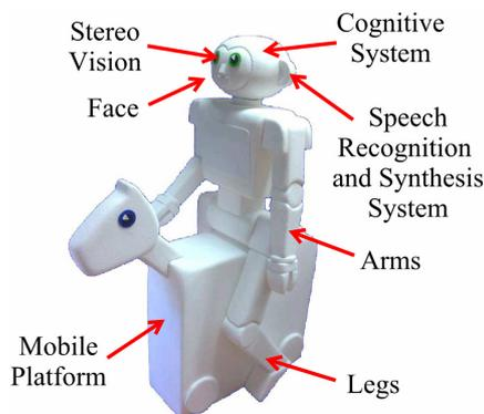
**Figure 1. Robot MARKO - concept**
