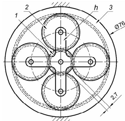
Figure 10. Scheme of the proposed planetary gearbox
