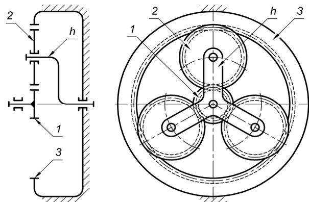
Figure 6. Planetary gearbox scheme
