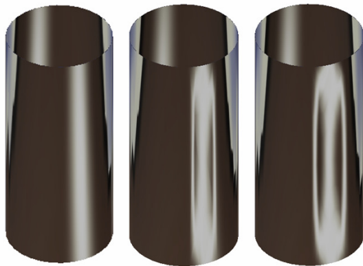
Figure 9 3D models of specimens (dent= 0mm, 2mm and 4mm, respectively)
