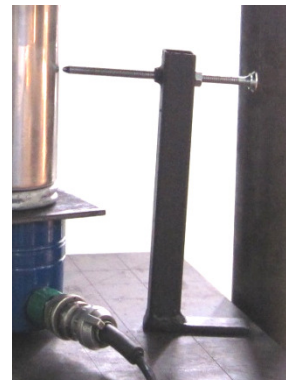
Figure 4. Mechanism for making dents
