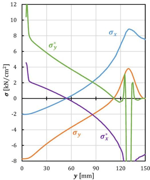
**Figure 5. Local stresses on upper flange ( $\sigma_x^*$ ,  $\sigma_y^*$ ) and lower flange ( $\sigma_x$ ,  $\sigma_y$ ) for  $R=0$**
