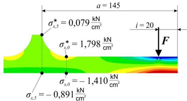
**Figure 6. Local stress state in longitudinal direction ( $R=27$  mm)**
