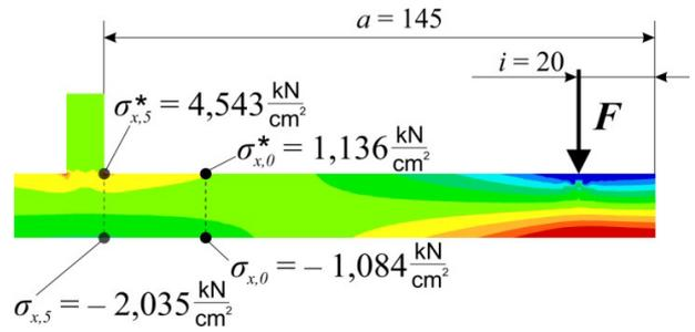
Figure 3. Local longitudinal stresses ( $R=0$ )
