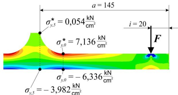
**Figure 7. Local stress state in transverse direction ( $R=27$  mm)**
