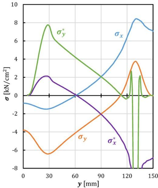
**Figure 8. Local stress state in the upper ( $\sigma_x^*$ ,  $\sigma_y^*$ ) and lower flange ( $\sigma_x$ ,  $\sigma_y$ ) for  $R=27$  mm**
