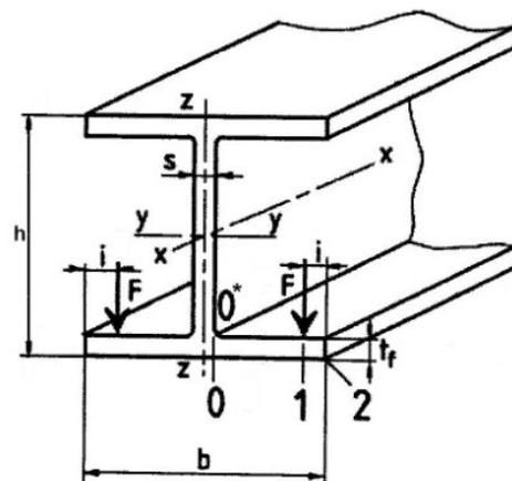
**Figure 1. Cross-section points, referent points and loads on parallel contour I-beam [1]**
