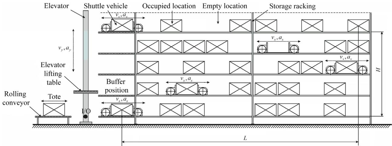
Figure 1. Tier-captive SBS/RS configuration – side view
