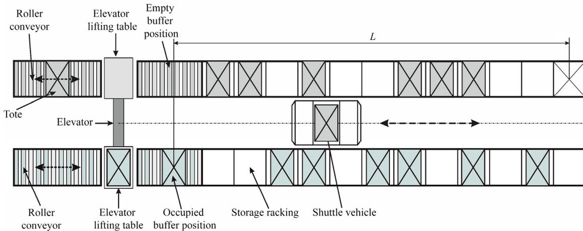
Figure 2. Tier-captive SBS/RS configuration – top view
