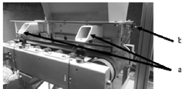
Figure 2. Test facility with load cells
