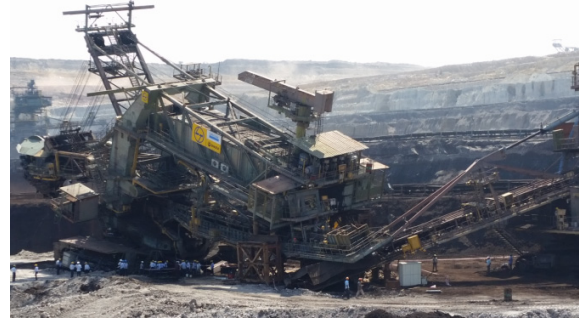
Figure 5. Catastrophic failure of the Bucket Wheel Excavator
