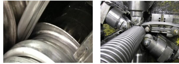
Figure 6. Manufacture process of carcass layer [41]
