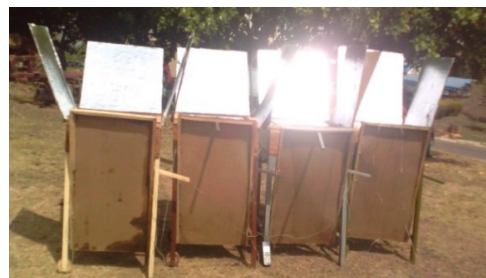
Figure 1b Experimental setup of DEBSCs with the base reflectors closed
