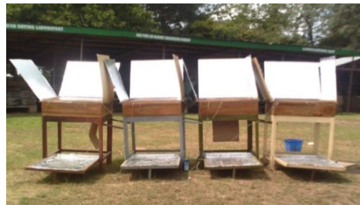
Figure 1a. Experimental setup of DEBSCs with the base reflectors exposed
