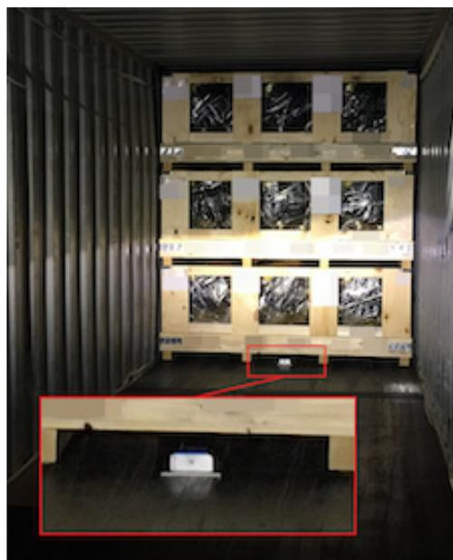
Figure 4. Position of data recorder in container
