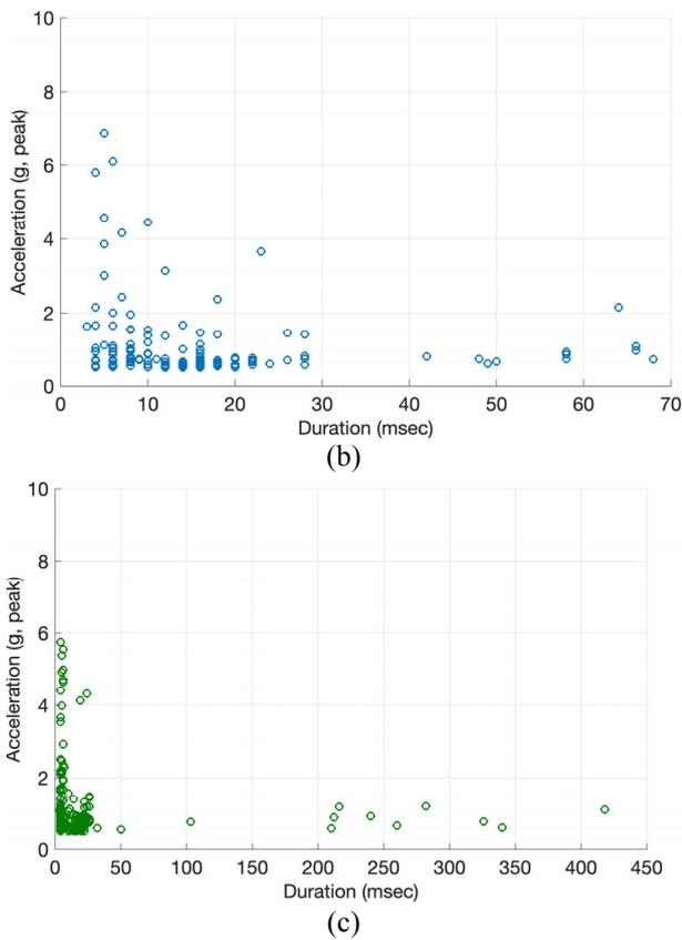
**Figure 9. Acceleration peaks versus pulse duration for all measured impacts in all three orientations a) vertical, b) lateral, and c) longitudinal**
