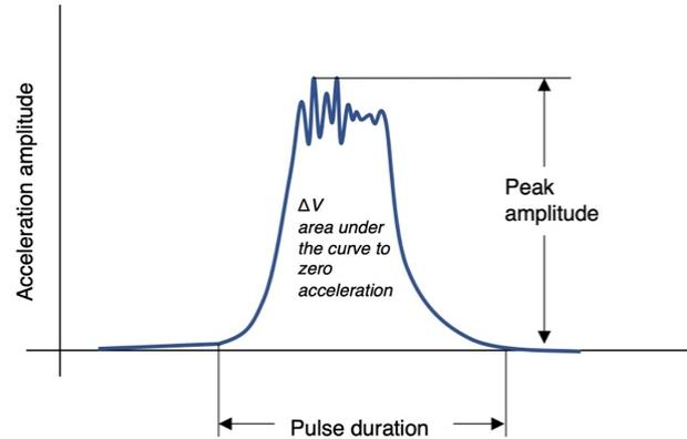
**Figure 6. Standard impact shock pulse with its components**
