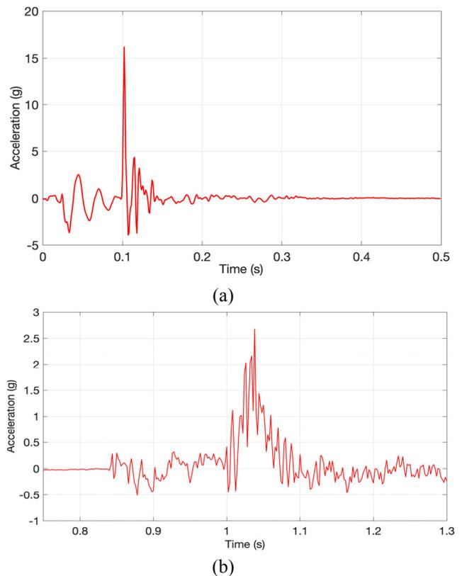
**Figure 8. Acceleration time histories for a) highest acceleration peak and b) highest velocity change**
