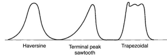
**Figure 7. Typical shock waveform shapes with cushioning [23]**
