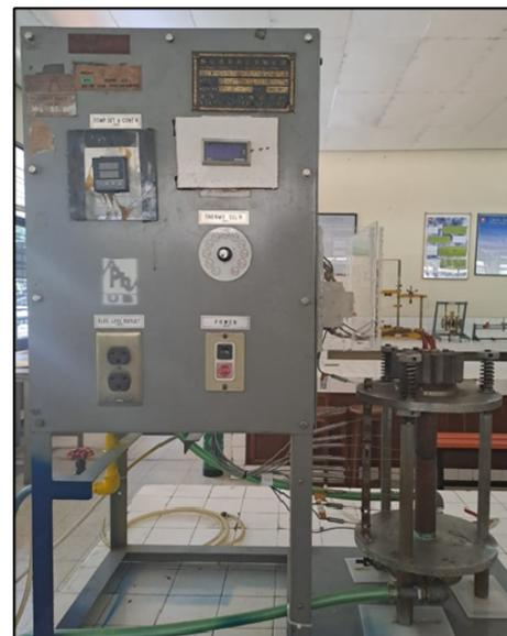
**Figure 5. Thermal conductivity measuring apparatus.**
