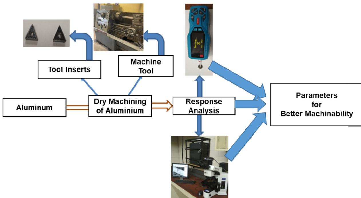
Figure 1. Process sequence to investigate dry machining of aluminum.
