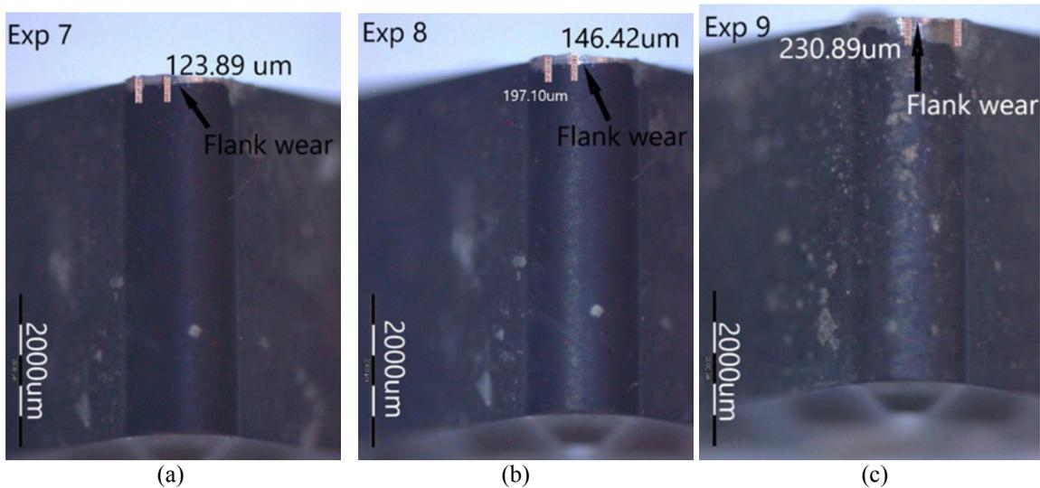
Figure 9. Flank wear on tool inserts during set 2 experiments 7 to 9
