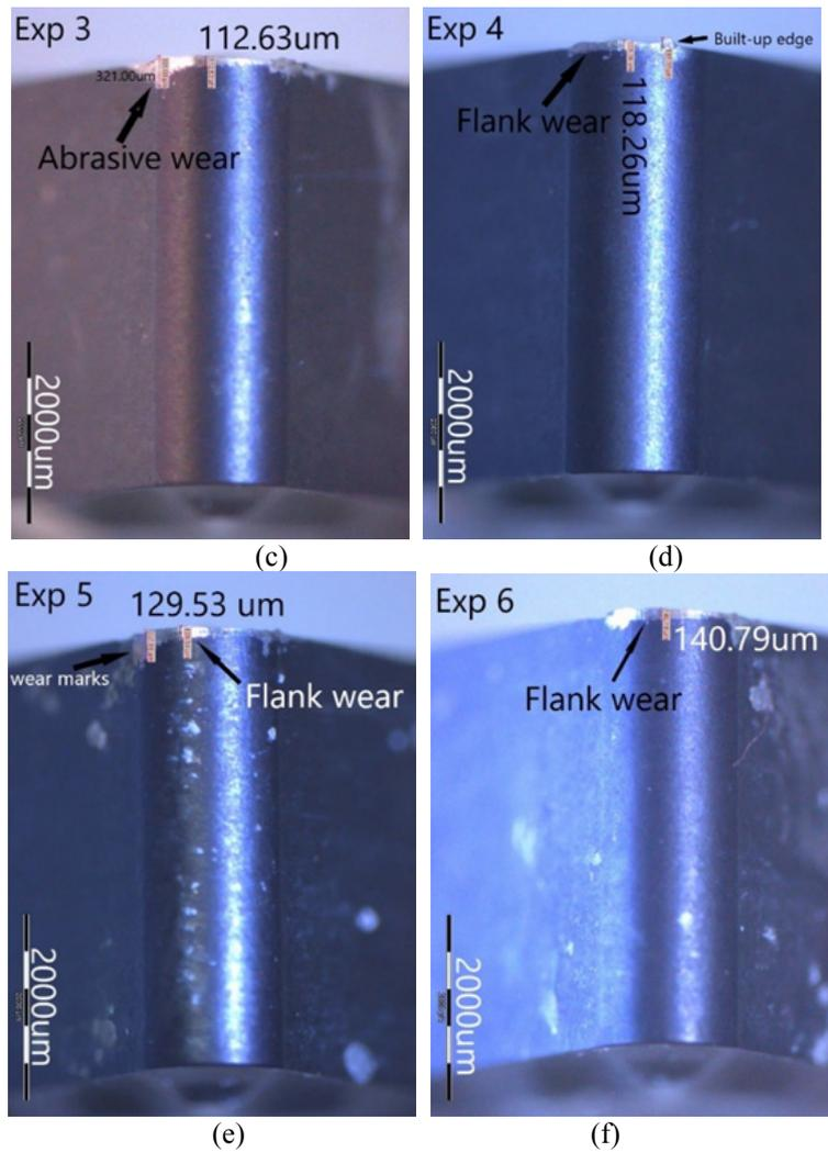
Figure 8. Flank wear on tool inserts during set 2 experiments 1 to 6
