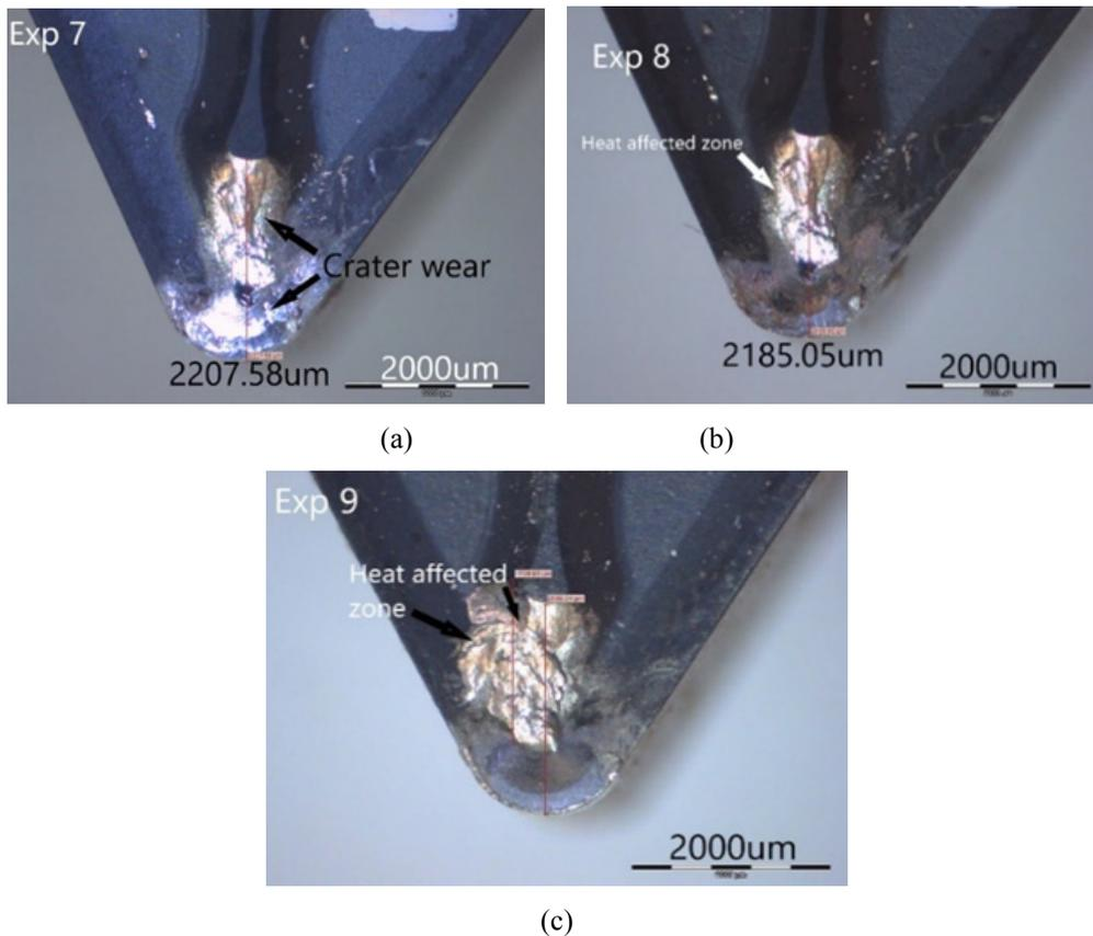
Figure 11. Crater wear on tool inserts during set 2 experiments 7 to 9
