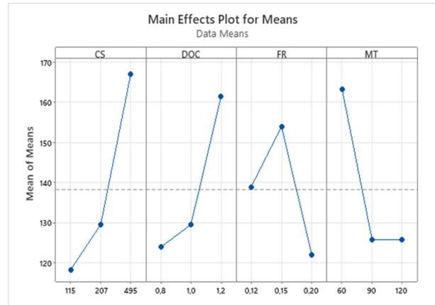
Figure 7. Main effect plots for flank wear vs CS, DOC, FR, MT
