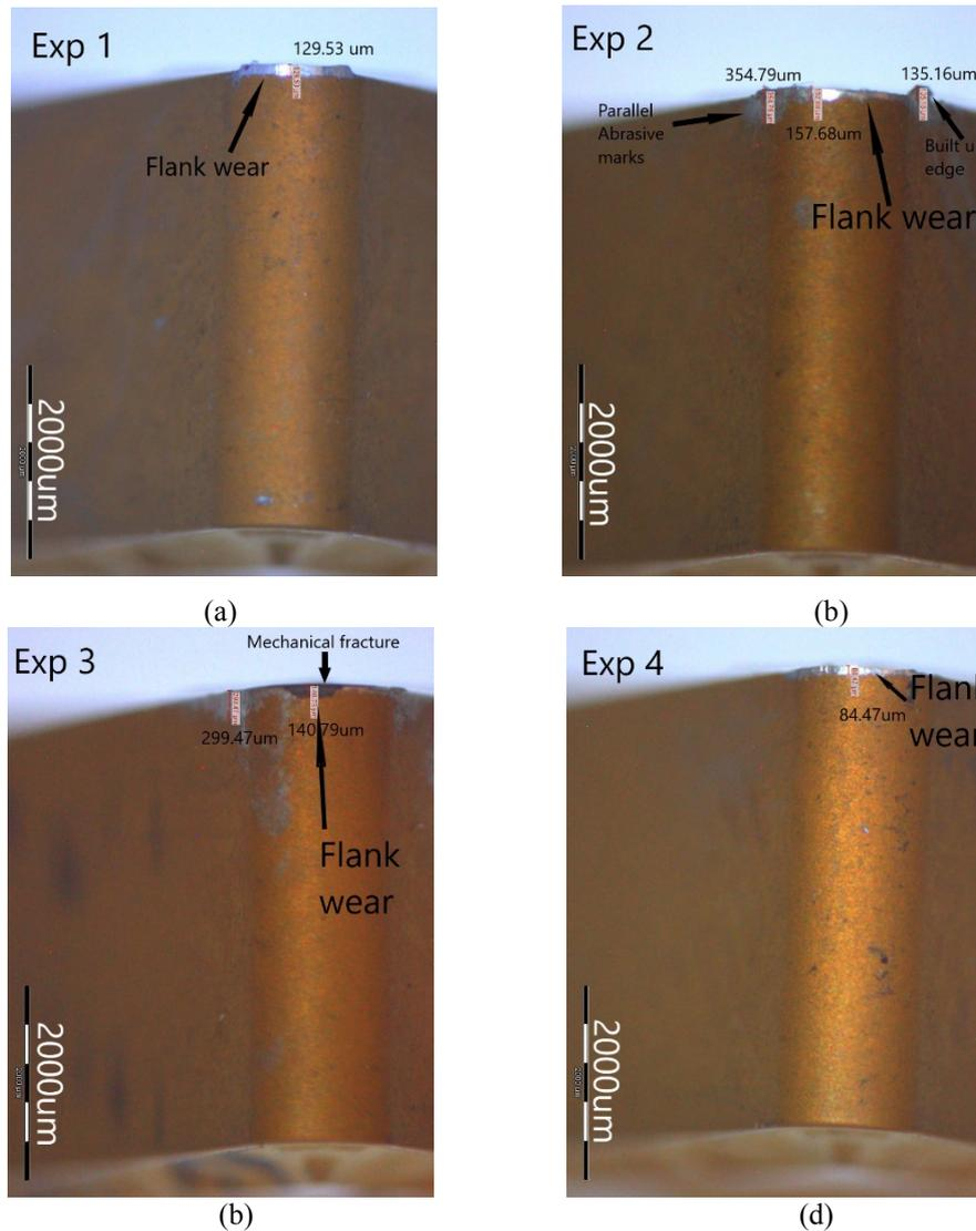
Figure 2. Flank wear on tool inserts during set 1 experiments
