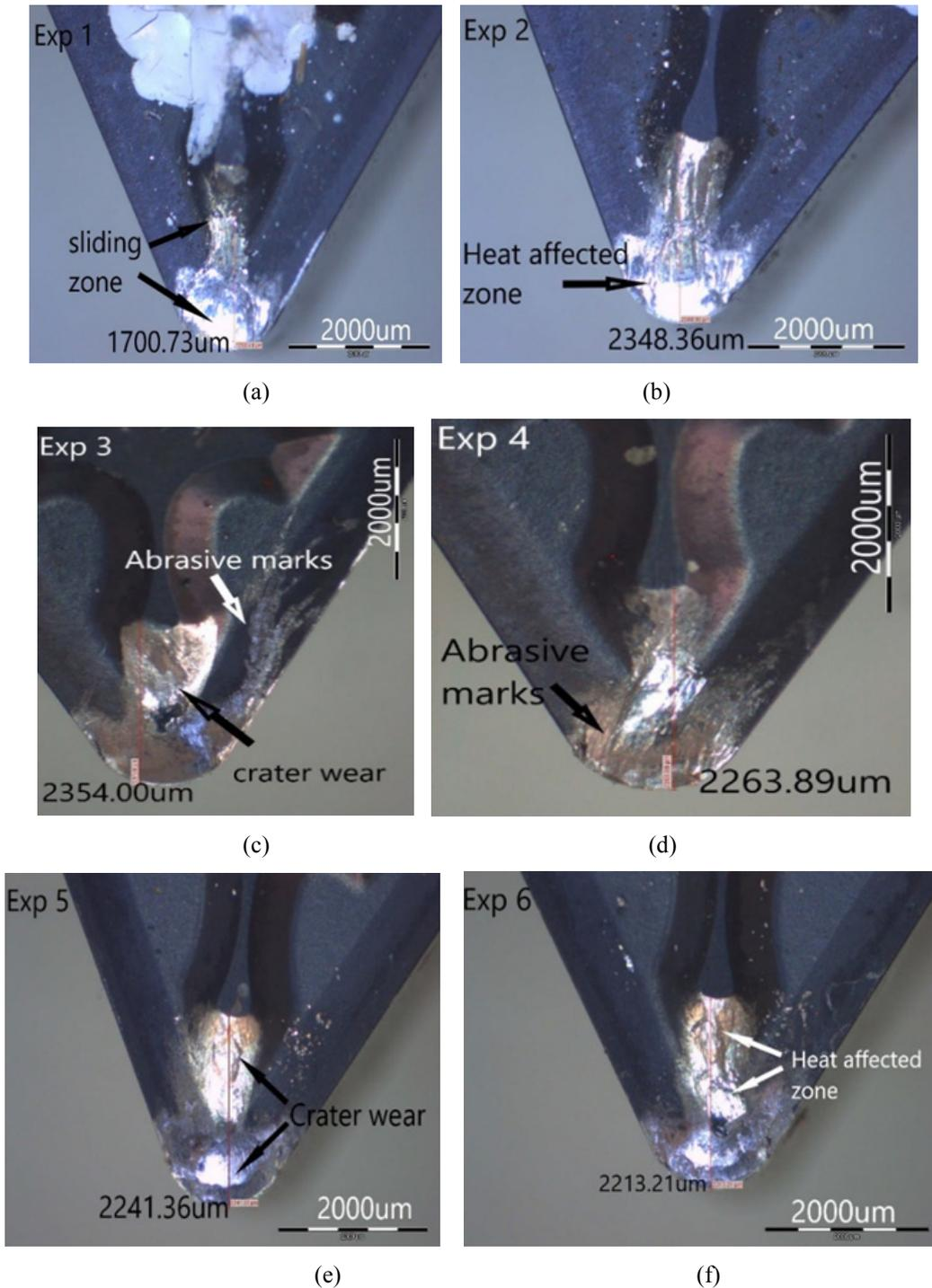
Figure 10. Crater wear on tool inserts during set 2 experiments 1 to 6
