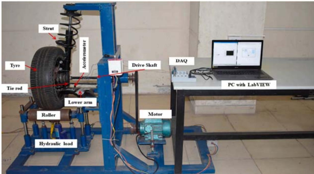
**Figure 1. Fabricated test setup**
