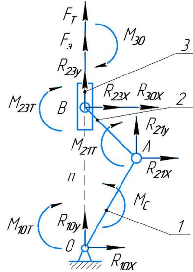
Figure 3. Mechanism diagram with applied forces and reactions in kinematic pairs
