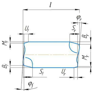
$\varphi$  – angle of work-pieces end;  $M$ ,  $U$  – cross and longitudinal dimensions of the tightening;  $B$ ,  $S$  – cross and longitudinal dimensions of the knife marks;  $f$ ,  $r$  – indexes indicating front and rear ends
