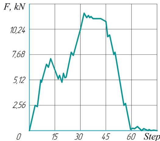
**Figure 5. Graph of the change in the cutting force during the separation of a tubular workpiece**
