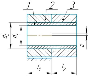
**Figure 4. The design diagram of the process of cutting off a measured tubular workpiece**
