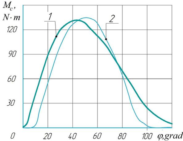
Figure 7. Dependence of the moment on the movable blade-bushing on the angle of rotation of the blade
