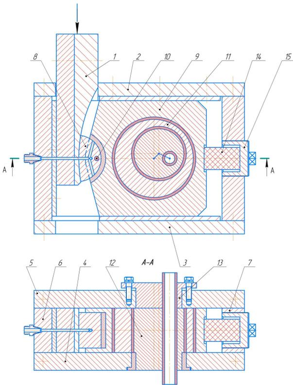
**Figure 10. Device for cutting pipes**
