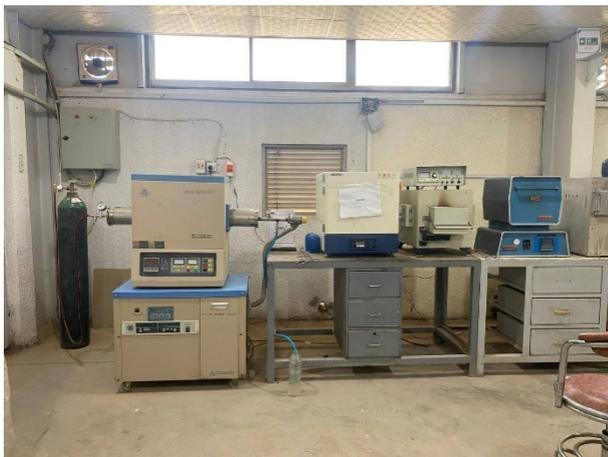
Figure 4. Sintering process (a) Sintering heat cycle (b) Tubler vacuuming furnace with an inert atmosphere.
