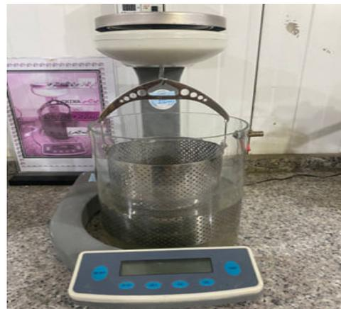
Figure 6. suspended mass and dry mass measurement
