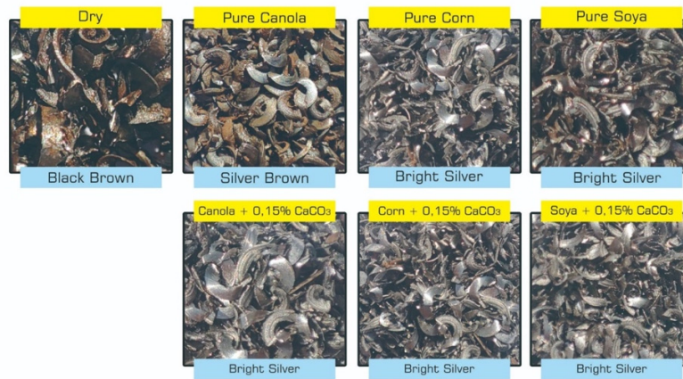
Fig 19. Chip Color in CNC Milling Process
