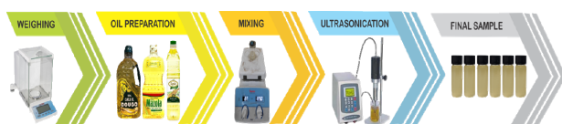
Fig 1. Process of Sample Nano-Cutting Fluid Preparation using a Two-Step Method
