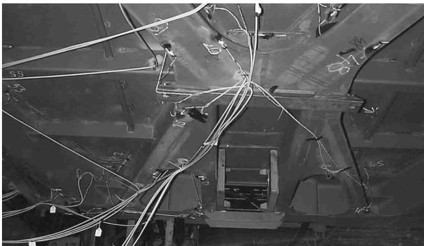
Figure 6. Headstock in the automatic coupling area with fitted strain gauges
