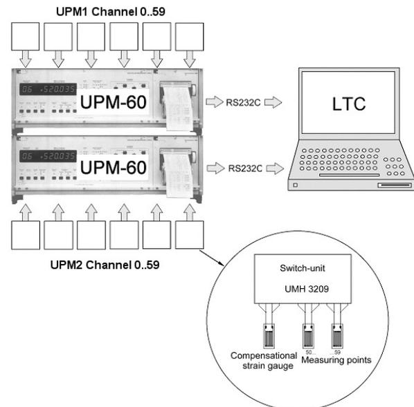
Figure 4. Principal scheme of the measuring chain
