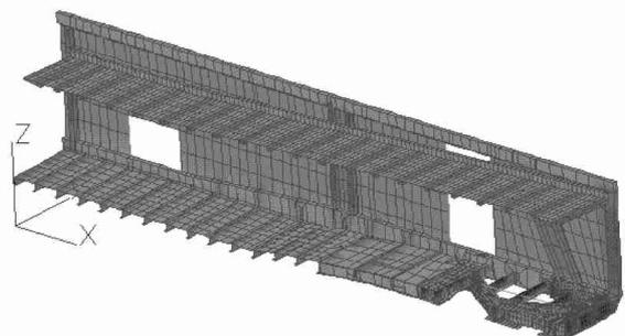
Figure 1. Model of wagon bearing structure
