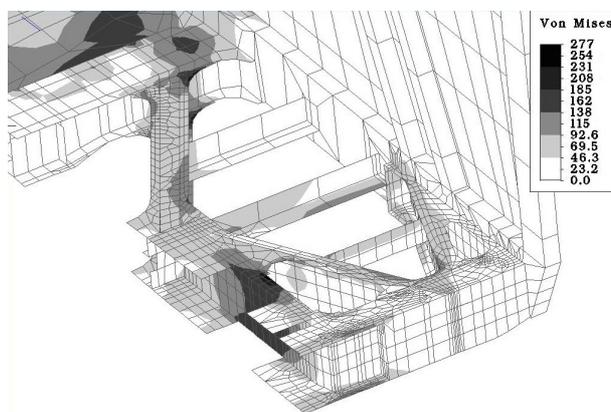
Figure 7. Stress distribution for load case 4 in headstock area.
