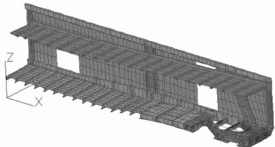
Figure 1. Model of wagon bearing structure
