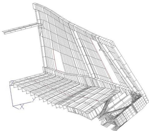
**Figure 8. Deformed structure in the case of torsional stiffness calculation.**
