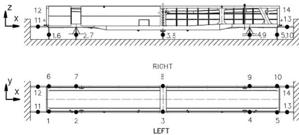
Figure 5. Arrangement of comparators
