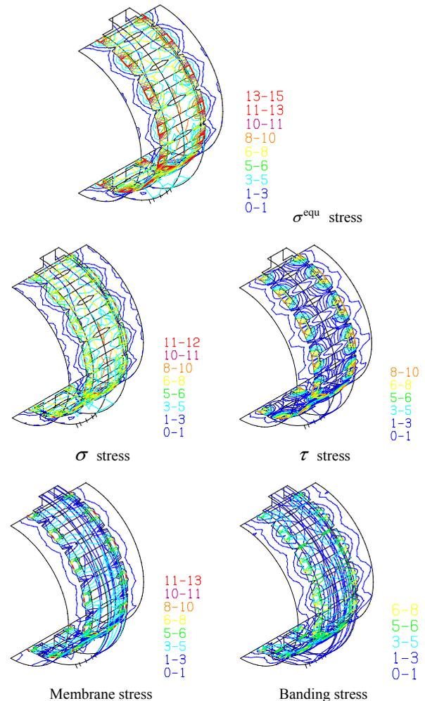
Figure 6. Equivalent stress field [ $\text{kN/cm}^2$ ]
