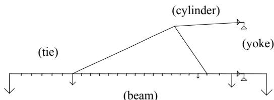
Figure 9. Planar model of the cantilever
