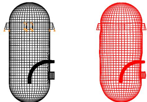
Figure 7. Model and deformation ( $f_{\max} = 0.24 \text{ cm}$ )
