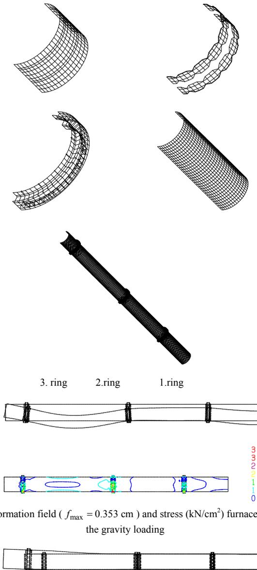
Figure 5. Model, deformation field ( $f_{\max} = 6.72 \text{ cm}$ ) and stress ( $\sigma_{\max}^{\text{equ}} = 15 \text{ kN/cm}^2$ ) furnace of the gravity-thermal loading ( $\Delta T = 100^\circ\text{C}$ )
