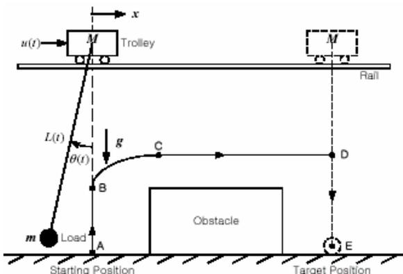
Figure 16. Path planning: Four stages of operation cycle
