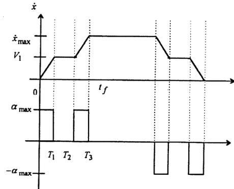
Figure 12. The stepped velocity pattern
