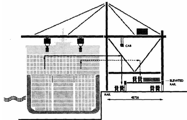
Figure 15. Crane system with double trolleys
