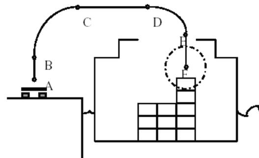
**Figure 4. A "desired" trajectory of container**
