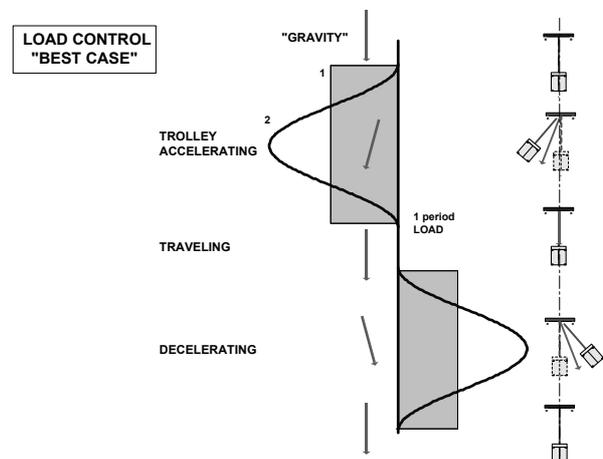
Figure 22. The "best" case of load control
