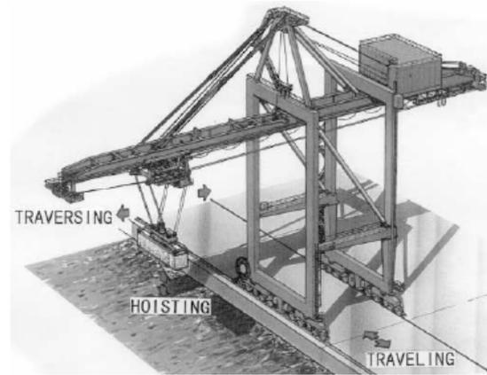
Figure 6. An outline of STS crane in operation
