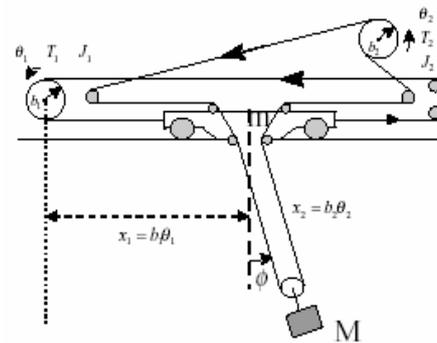
Figure 7. First simplification of trolley model
