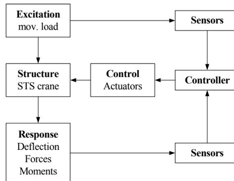
Figure 18. Block diagram of structural control problem
