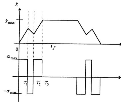
Figure 13. The notched velocity pattern
