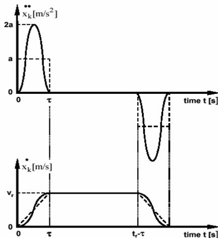
Figure 11. The modification of standard trapezoidal velocity pattern
