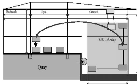
**Figure 3. Schematical drawing of crane operation**
