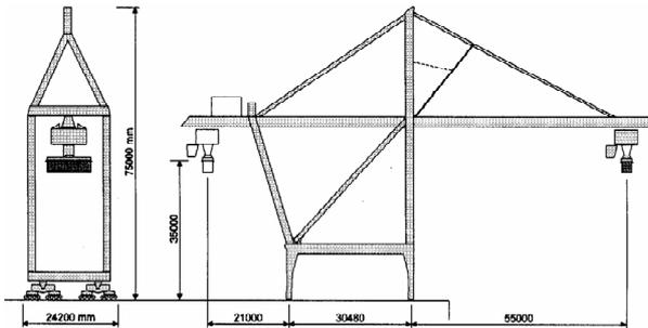
Figure 19. Rigid structure mega crane by Mitsubishi Heavy Industries
