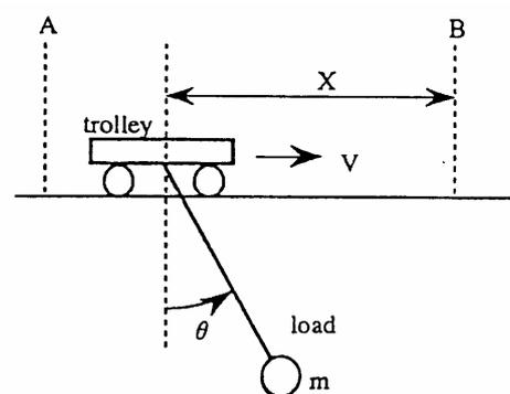
Figure 8. Final simplification of trolley model
