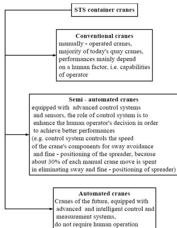
Figure 5. Classification of cranes by their degree of automation
