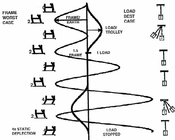
Figure 23. Dynamic interaction load - structure
