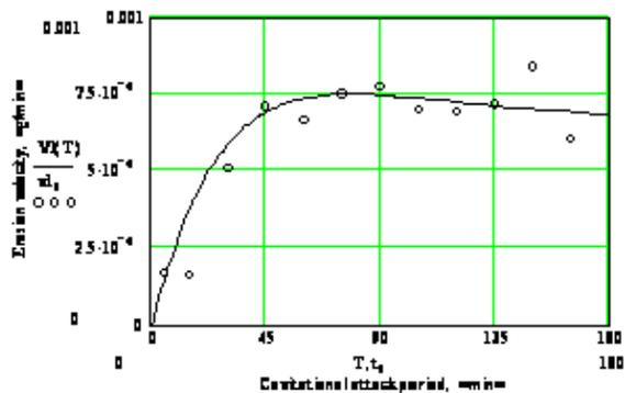
Figure3. Erosion velocity for OL 370-3k
