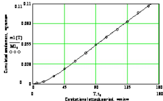
Figure 2. Eroded mass OL 370-3k
