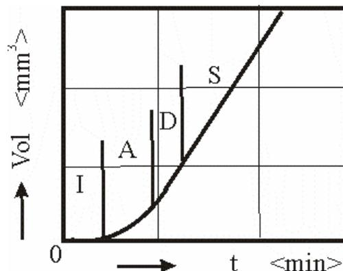
Figure1a. The typical cavitation erosion curves (volumetric losses  $Vol(t)$ )
