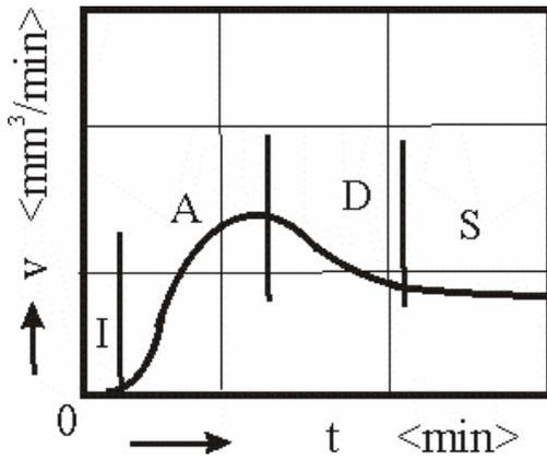
Figure 1b. The typical cavitation erosion curves (erosion velocity  $v(t)$ )
