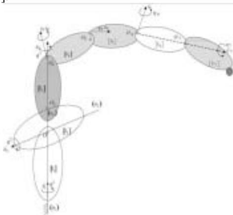
Figure 9. Upper limb model as open linkage with 7 DOF-joints
