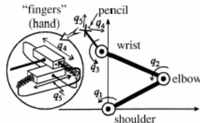
Figure 13. Configuration of the writing mechanism: five-DOFs planar arm
