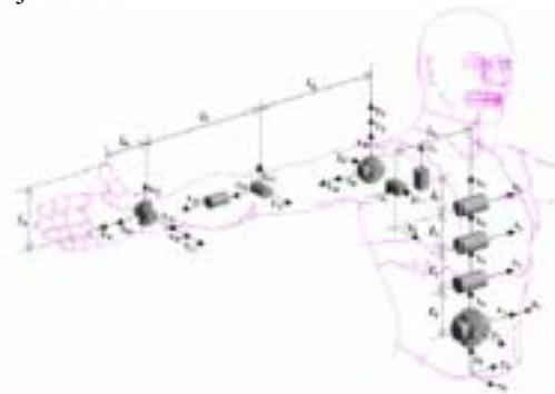
Figure 11. Modeling of the torso-right shoulder arm
