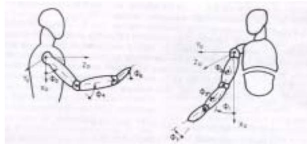
Figure 10. The general coordinates  $q_i$  associated with the terms for motions in the gross joints accepted in anatomy
