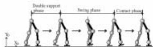
Figure 8. Three walking phases
