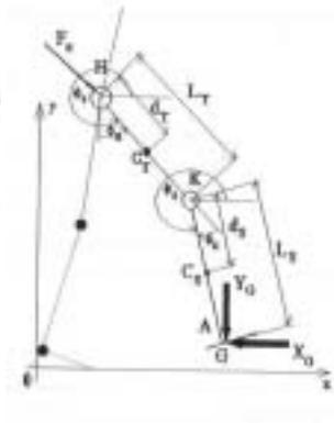
Figure 7b. Model of the two-link skeleton
