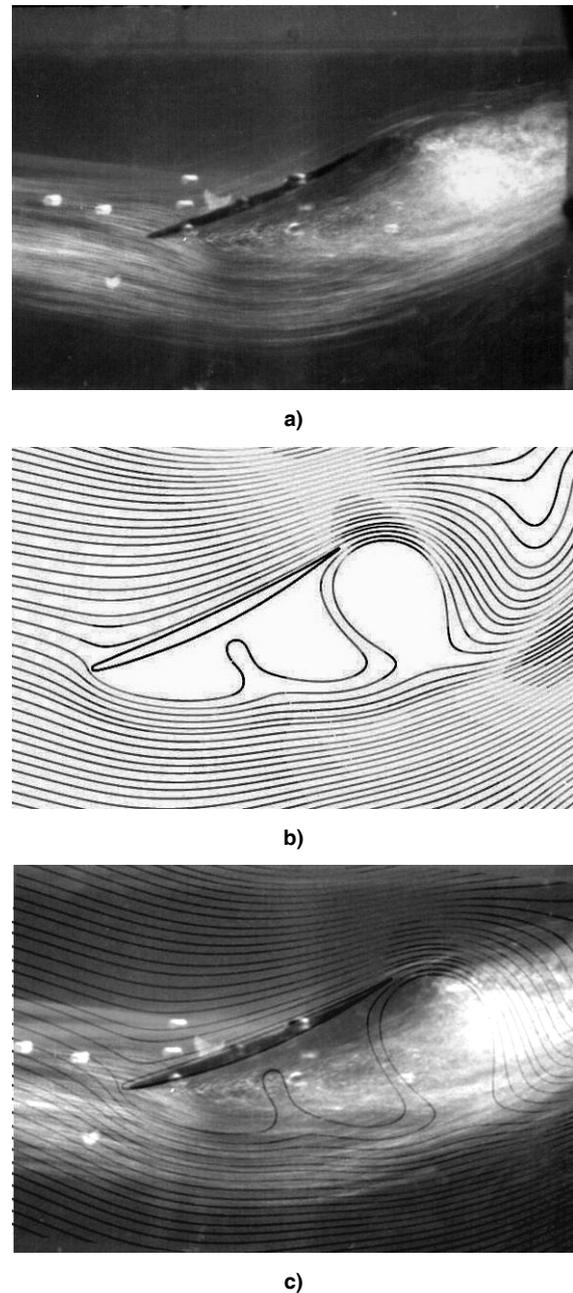
Figure 5. Flow visualization around hydroprofile for  $V_\infty = 3$  m/s ; (a) air bubbles, (b) visualization of numerical data, (c) composite visualization .
