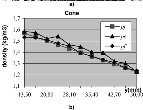
Figure 3. Simultaneous presentation of experimntal and numerical flow around cone  $M_\infty = 1.71$  (a) and density distribution behind shock wave for  $x = 50$  mm (b)
