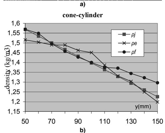
Figure 4. Simultaneous presentation of experimental and numerical flow around cone-cylinder for  $M_\infty = 1.474$  (a) and density distribution behind shock wave for  $x = 150$  mm (b)
