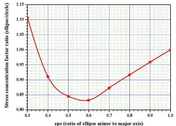
**Figure 4. Elliptical star tip calculation results**
