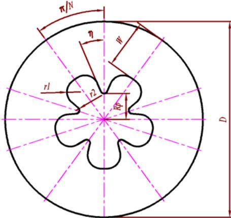
**Figure 1. Cross section of existing propellant grain**
