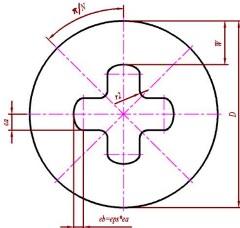
**Figure 2. Cross section of improved propellant grain**
