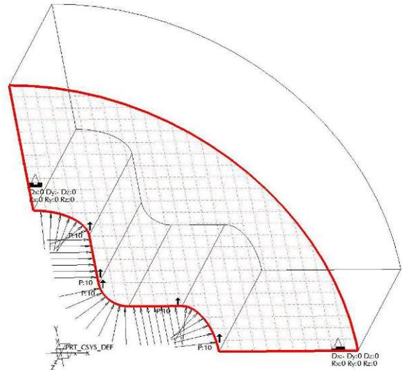
**Figure 3. Pro/Mechanica simulation model**
