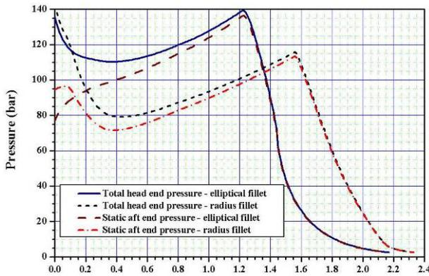
**Figure 9. Pressure vs. time comparison between old and new design with higher burning rate propellant**
