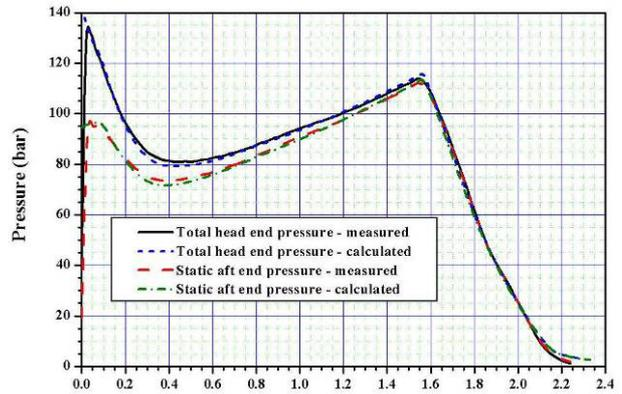
Figure 5. Pressure vs. time history for old star shape grain
