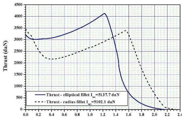
**Figure 10. Thrust vs. time comparison between old and new design with higher burning rate propellant**
