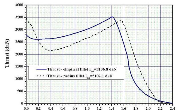
Figure 8. Thrust vs. time comparison between old and new design
