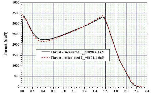
Figure 6. Thrust vs. time history for old star shape grain
