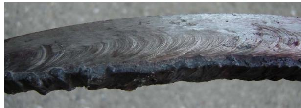
Figure 3. Pores at the inner side of flange
