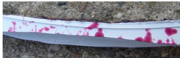
Figure 4. Cracks in a flange welded joint
