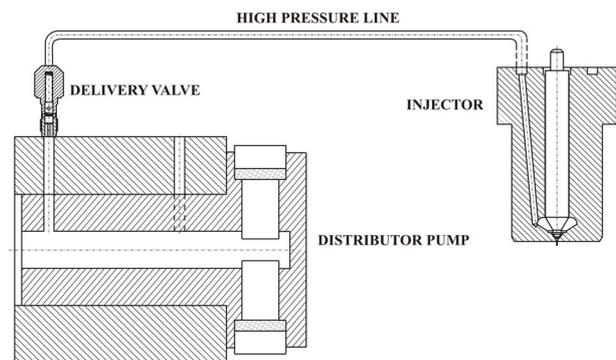
**Figure 1. Fuel injection system with the piston-radial distributor pump**
