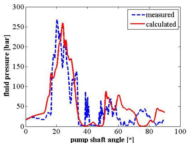
Figure 3. The comparison of measured and calculated fluid pressure at the end of the high pressure line
