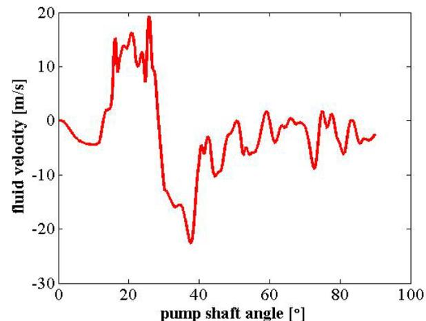
Figure 4. The change in fluid velocity at the end of the high pressure line
