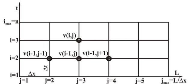
Figure 2. Calculation scheme for fluid velocity along the high pressure line
