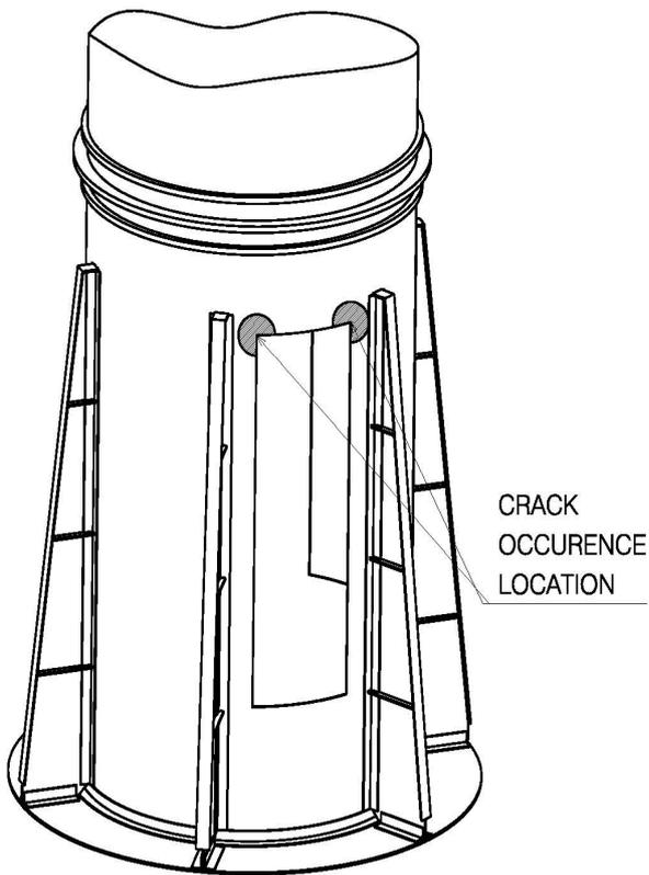
Figure 3. Chimney's root section
