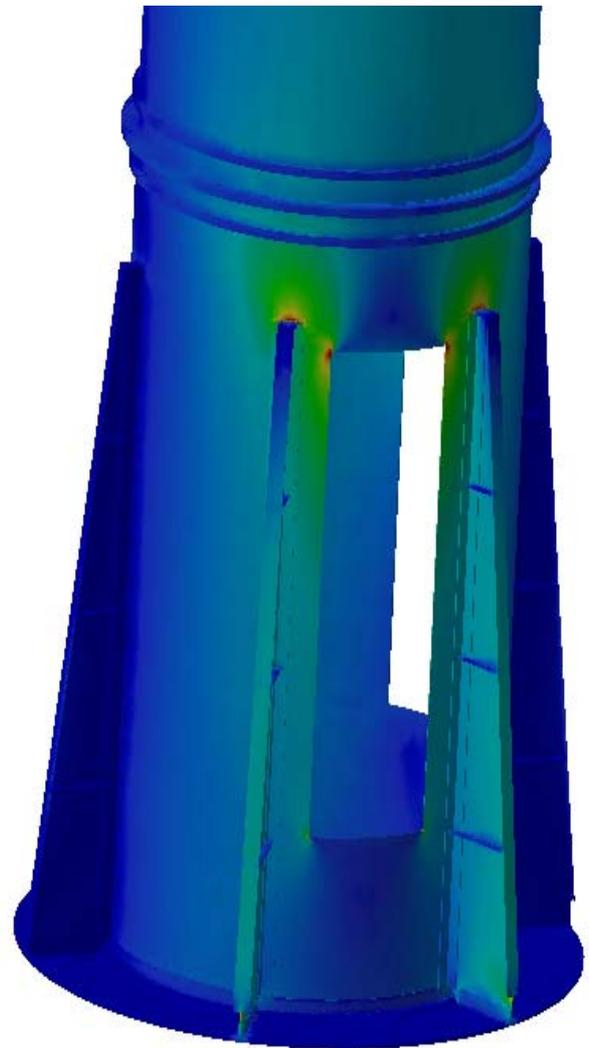
Figure 11. Uniaxial stress field on the chimney's root segment
