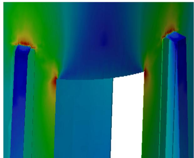
Figure 12. Distribution of the uniaxial stress at the zone of flue duct upper corners
