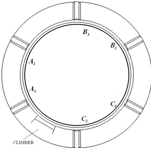
Figure 4. Top view of cracks dispositions
