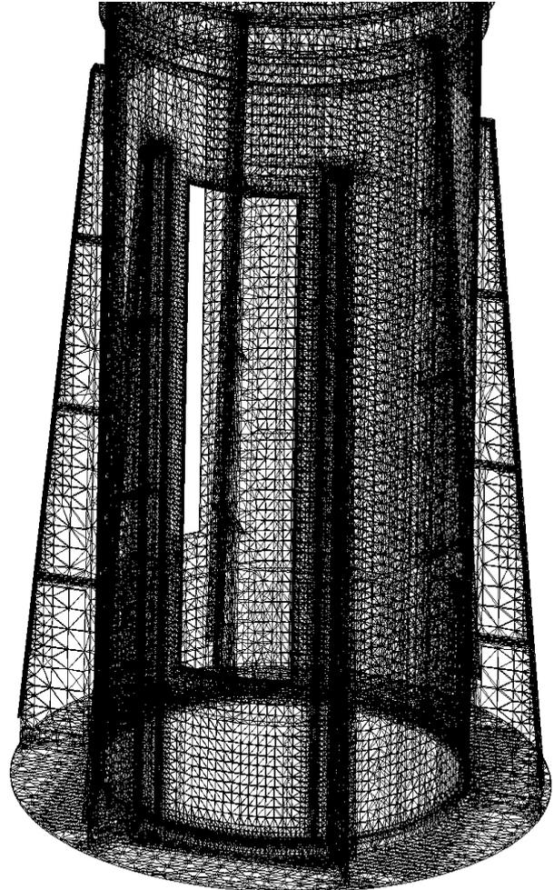
Figure 9. FEM Model of chimney's root section
